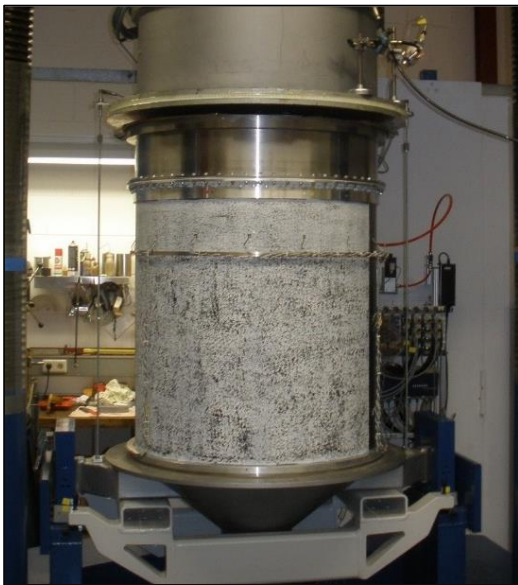
Figure 6 – Buckling tests including VCT measurement with the same samples at 2 different test facilities [8]
