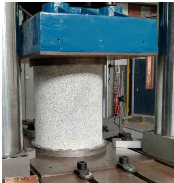
Figure 6 – Buckling tests including VCT measurement with the same samples at 2 different test facilities [8]
