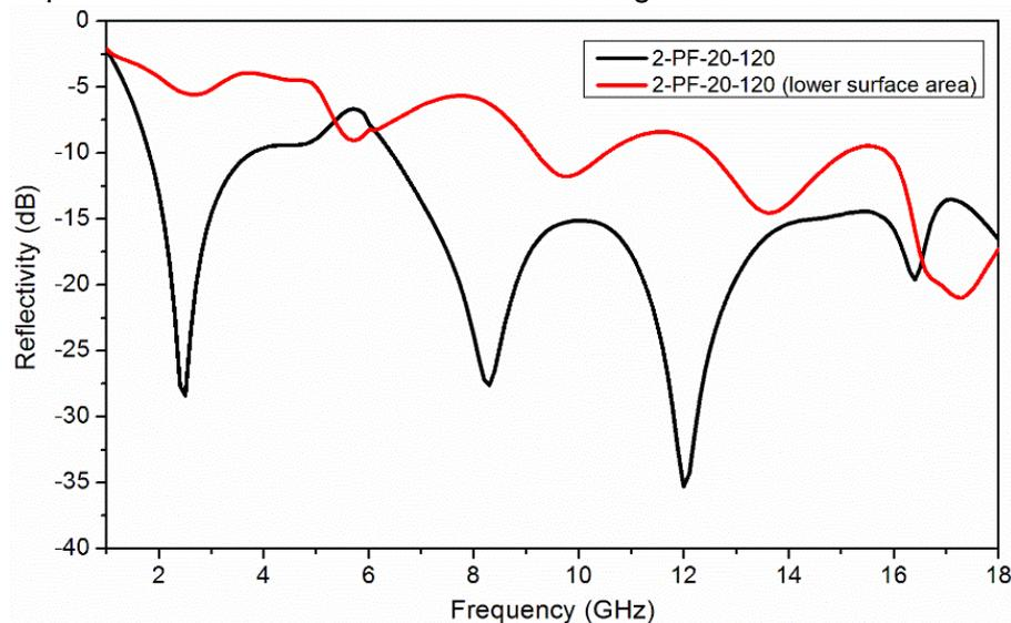
Figure 3 The influence of surface area of active carbon on the reflectivity of MAHCMs
