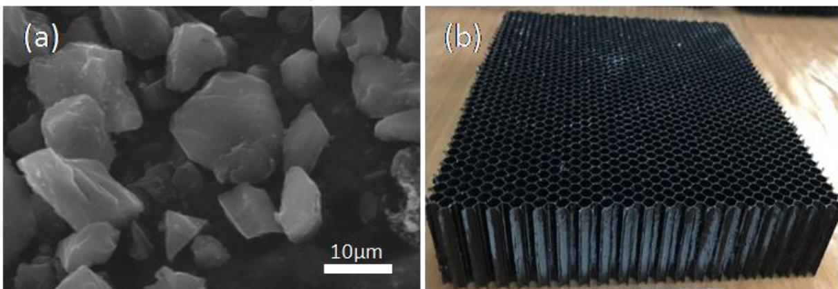
Figure 2 (a) The micro-morphology of active carbon and (b) the picture of MAHCM
