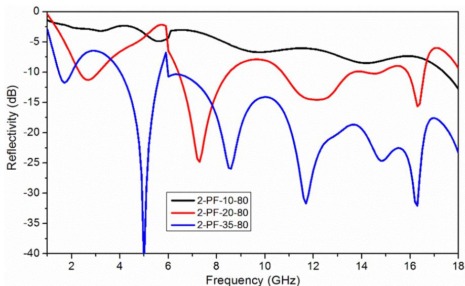
Figure 4 The influence of the thickness of honeycomb on the reflectivity of MAHCMs
