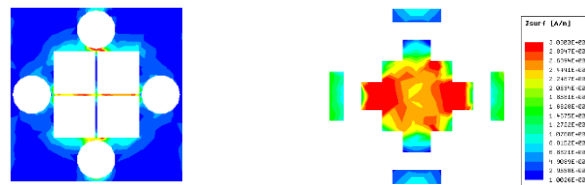
(a) Transmission functional layer (b) Absorbing functional layer Figure 12 –The surface current distribution. (11.5GHz)
