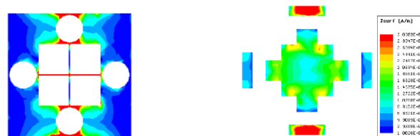
(a) Transmission functional layer (b) Absorbing functional layer Figure 13 –The surface current distribution. (18.0GHz)
