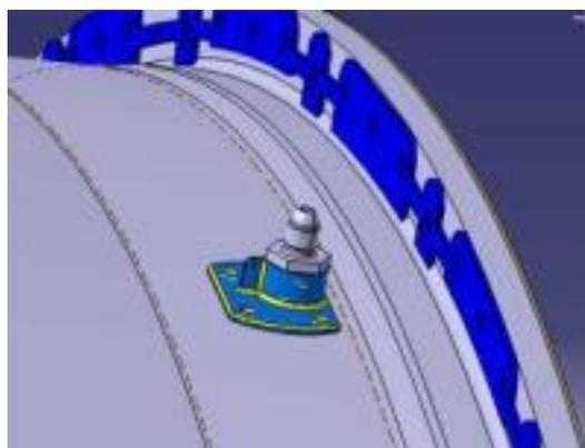
Figure 3 – The static pressure data PS12 at the fan inlet
