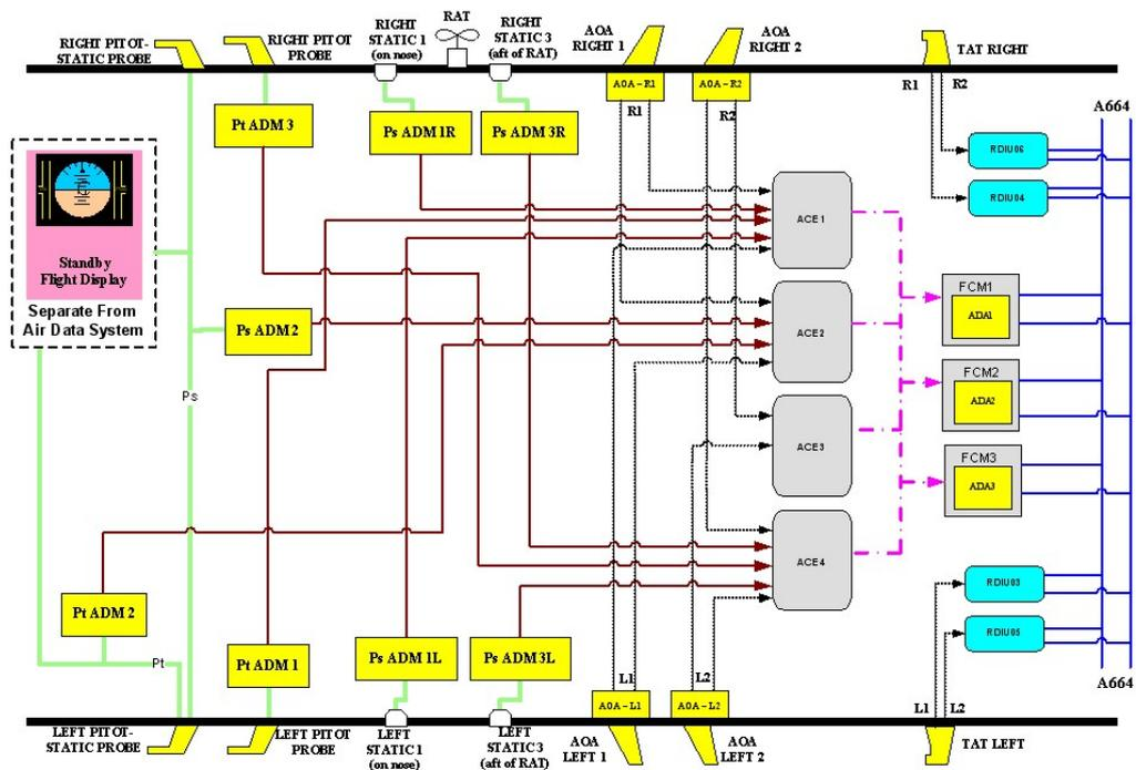
Figure 2 – Aircraft air data system principle diagram
