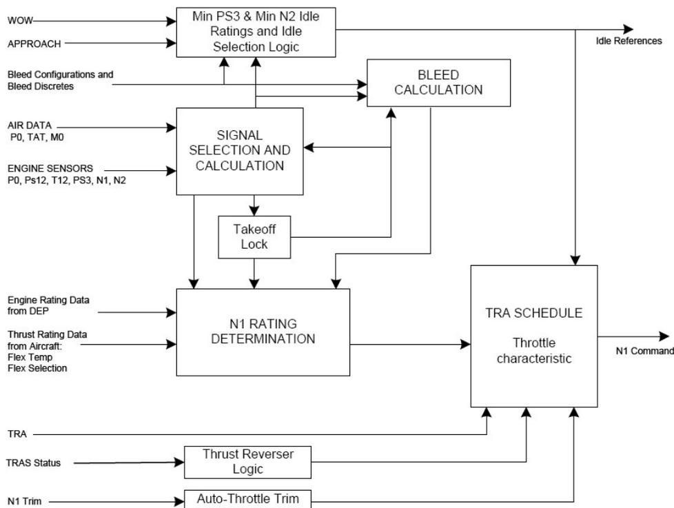
Figure 1 – Engine power management principle diagram.
