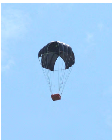
Fig. 1 : Steerable cruciform parachute system during outdoor flight-testing
