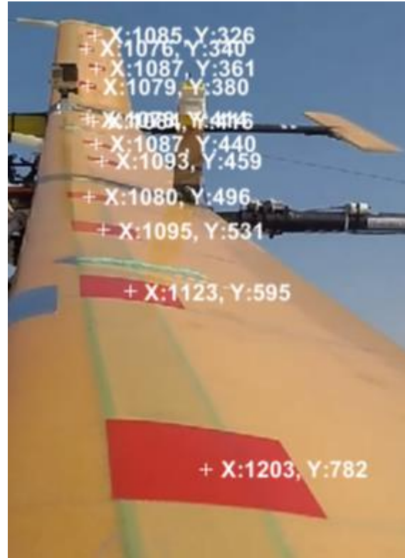
Fig. 4. Image coordinates acquired through the red object detection algorithm.
