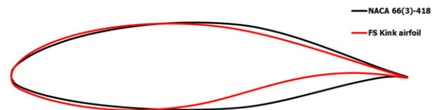
Fig. 7 Kink airfoil: comparison with the reference NACA laminar airfoil.
