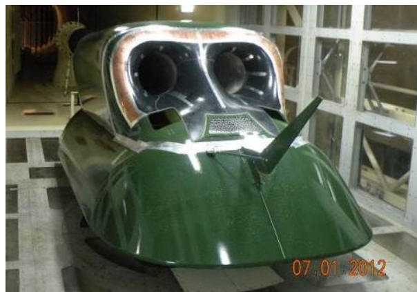
Fig. 1: Thermal intake model in IWT
