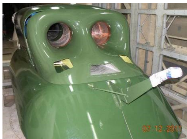
Fig. 2: Aerodynamic intake model in IWT
