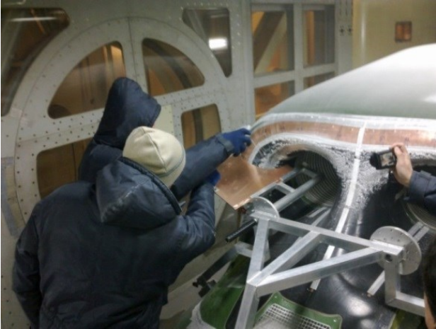
Fig. 23: Ice accretion measurements, directly after the ice test
