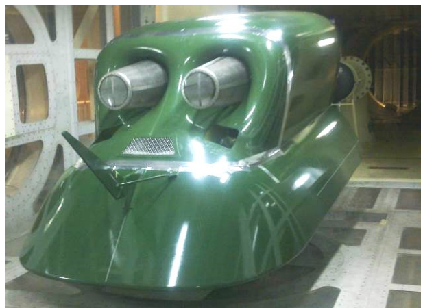
Fig. 6: Model with passive IPS screens in IWT
