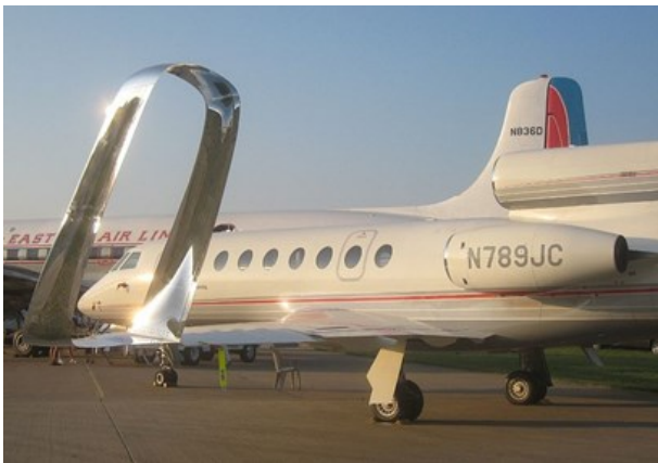
Fig. 9. Biplane winglet of the Gulf Stream airplane.
