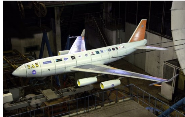
Fig. 3. Dynamically-scaled model (EURAM) with external (remote) aileron
