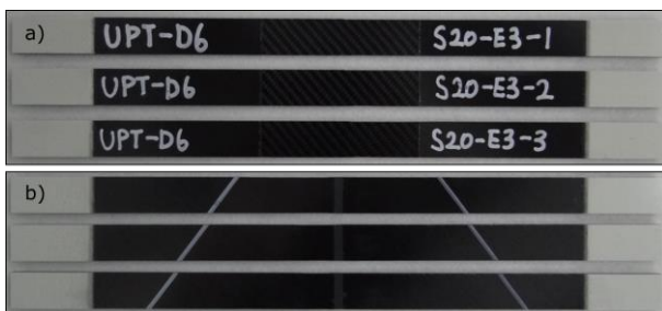
Fig. 1. Schematic configuration of repaired laminate used for tensile testing.
