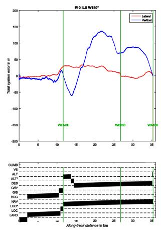
Figure 4 ILS W180 from 23 July 2015. The top panel shows lateral and vertical flight technical error, the bottom panel indicates autopilot modes active during the approach. Green lines mark the approach waypoints. The dive and drive mode is visible in the vertical modes from kilometer 12 to 15 and in the vertical FTE variation between WFCAF and WB180.
