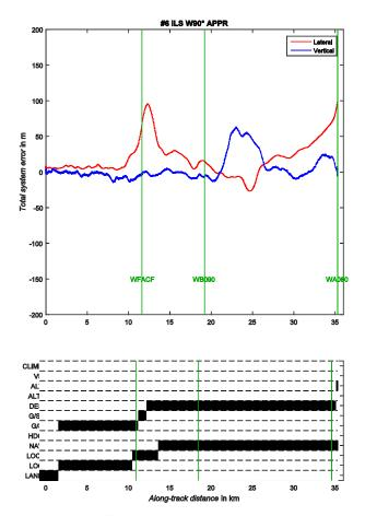
Figure 5 ILS W90 from 20 July 2015 with the approach mode armed at WA090. The top panel shows lateral and vertical flight technical error, the bottom panel indicates autopilot modes active during the approach. Green lines mark the approach waypoints. The cross track error spike slightly before WFACF is caused by early intercept of the localizer.
