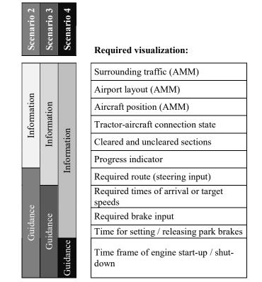
Fig. 5. Required Functions of the HMI Pending the Mode of Automation (Scenarios)
