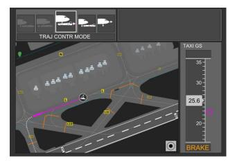
Fig. 6. Conceptual HMI Design for an EFB (AMM Source: Gate-to-Gate Application of Jeppesen GmbH)
