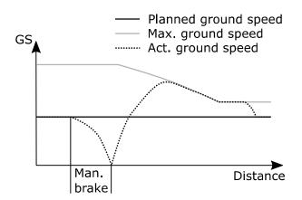
Fig. 3. Ground Speed (GS) Set by Tractor's Control Loop after Manual Braking Input
