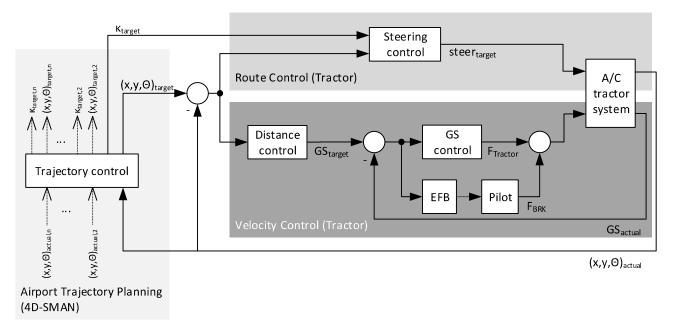
Fig. 4. Schematic Design for Proposed Trajectory Control Loop
