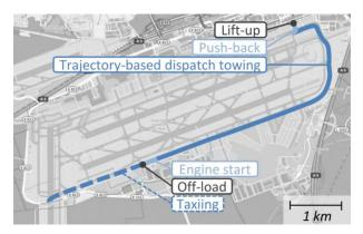
Fig. 2. Exemplary Route for Automated Dispatch Towing Operations at FRA (Map Source: openstreetmap.org)
