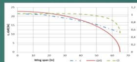
We divided the wing into 4 root sections available for twisting geometrically and aerodynamically. Because of different chords along wing span, there are different Reynolds numbers in each section. For that reason current airfoil had to be re-designed to meet requirements for smaller Reynolds numbers.
