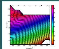
C++ code calculated the potential lift of a plane with a given wing area and span at certain take off distance with the formulas from Flight Mechanics including equation of motion:
