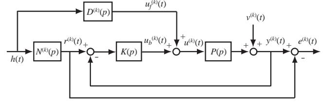
**Fig. 1** An iterative learning control system (ILCS) for identification.
