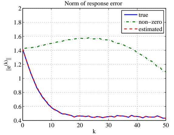
**Fig. 4** Norm of response error using three kinds of impulse responses in Case 1.
