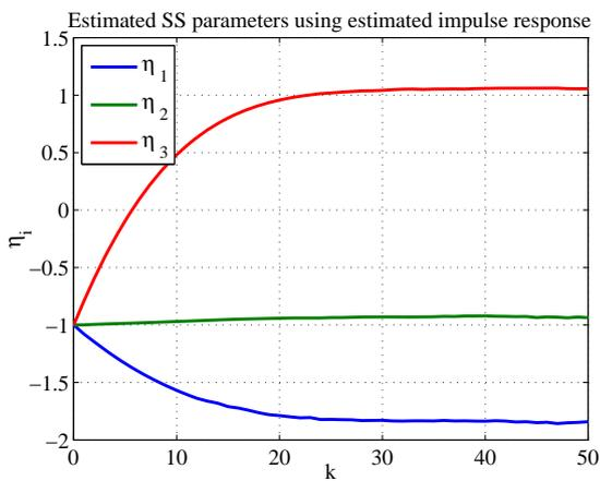
**Fig. 7** Estimated SS parameters using “estimated” impulse response in Case 1.
