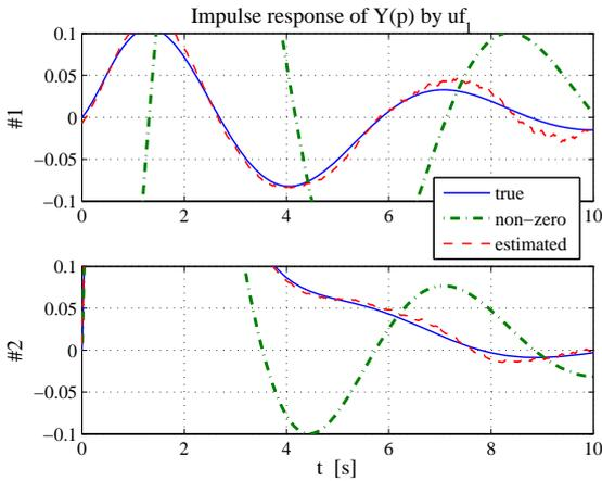
**Fig. 3** Impulse response of  $Y(p)$  by  $u_{f1}(t)$ .
