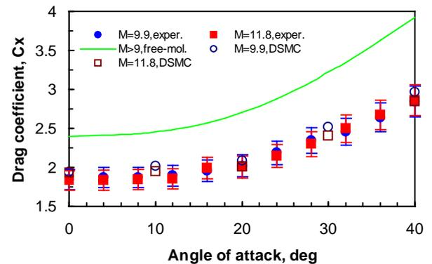
Fig. 10 Drag coefficient  $c_x$  of the wedge ( $2\theta = 40$  deg) at  $Re_0 = 4$  and various Mach numbers  $M_\infty$ .
