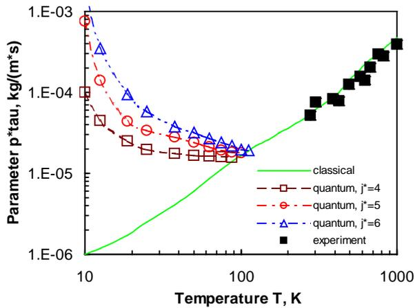
**Fig. 5** Relaxation time  $\tau_R$  of molecular nitrogen vs. kinetic temperature  $T_t$ : solid line - Parker's model [23]; open symbols - quantum rotational levels  $j^* = 4, 5,$  and  $6$  [21]. Experimental data from Refs. 24-25.
