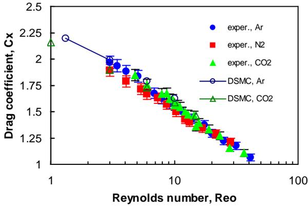
Fig. 12 Drag coefficient  $c_x$  of the wedge ( $2\theta = 40$  deg) for various gases vs. the Reynolds number  $Re_0$ .
