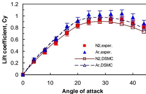
Fig. 13 Lift coefficient  $c_y$  of the wedge ( $2\theta = 40$  deg) at  $Re_0 = 3$  and various gases.
