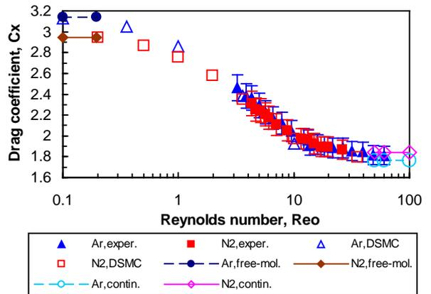
Fig. 15 Drag coefficient  $c_x$  of the plate at  $\alpha = 90$  deg for argon and nitrogen vs. the Reynolds number  $Re_0$ .
