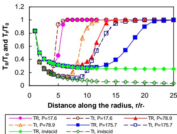
Fig. 7 Rotational  $T_R$  and translational  $T_t$  temperatures in spherical flow at different pressure ratios  $P$ .
