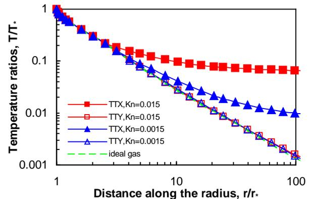
Fig. 4 Parallel ( $TTX$ ) and transverse ( $TTY$ ) temperature distributions in the spherical expansion of argon into vacuum at  $Kn^* = 0.015$  and  $0.0015$ .
