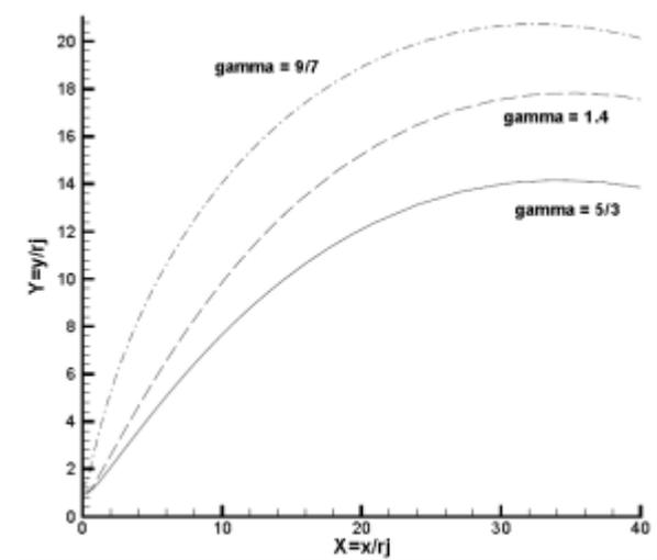
Fig. 2 Barrel shocks of inviscid axisymmetric jets for various gases at pressure ratio  $p_0/p_a = 1000$ .
