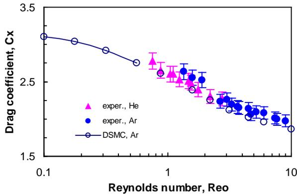
Fig. 16 Drag coefficient  $c_x$  of the plate at  $\alpha = 90$  deg in helium and argon vs. the Reynolds number  $Re_0$ .
