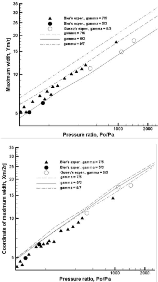
Fig. 3 *Top*: The maximum width  $Y_m = y_m/r_j$  of inviscid axisymmetric jets ( $M_j = 1$ ) for gases with different  $\gamma$  and at various pressure ratios  $p_0/p_a$ . *Bottom*: The axis coordinate  $x_m$  of the width  $y_m$ .
