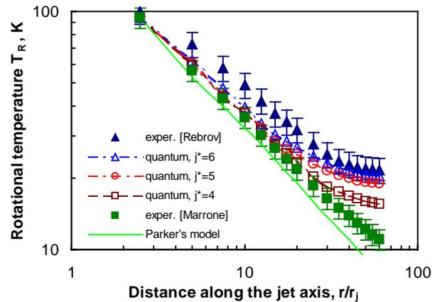
**Fig. 6** Rotational temperature  $T_R$  along the axis of nitrogen jet. Experimental data from Refs. 19-20.
