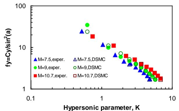
Fig. 9 Modified lift coefficient vs. hypersonic parameter  $K$  for the blunt plate ( $\delta = 0.06$ ).
