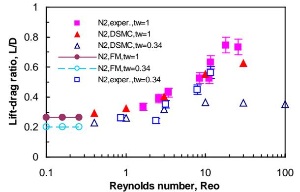
Fig. 17 Lift-drag ratio for the blunt plate ( $\delta = 0.1$ ) vs. Reynolds number  $Re_0$  in nitrogen at  $\alpha = 20$  deg and various temperature factors.
