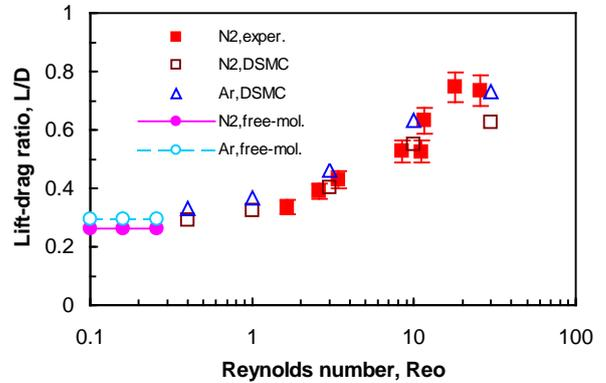
Fig. 14 Lift-drag ratio of the blunt plate ( $\delta = 0.1$ ) at  $\alpha = 20$  deg in Ar and N<sub>2</sub> vs. Reynolds number  $Re_0$ .
