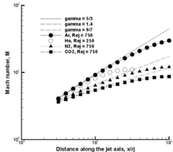
Fig. 1 Mach number  $M$  along the axis of axisymmetric jets of argon, helium, nitrogen, and carbonic acid.
