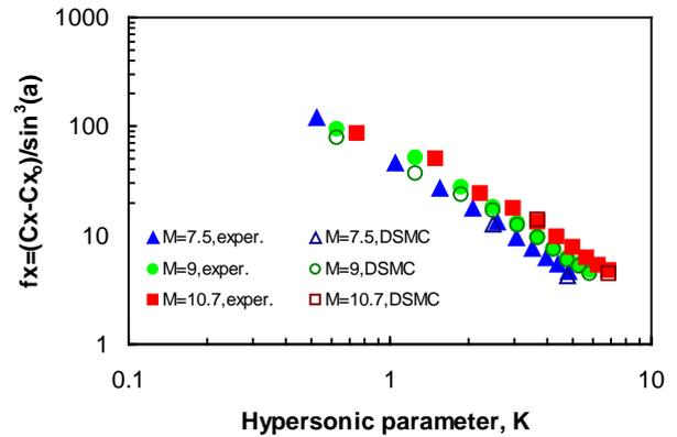
Fig. 8 Modified drag coefficient vs. hypersonic parameter  $K$  for the blunt plate ( $\delta = 0.06$ ).
