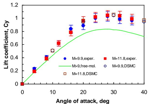
Fig. 11 Lift coefficient  $c_y$  of the wedge ( $2\theta = 40$  deg) at  $Re_0 = 4$  and various Mach numbers  $M_\infty$ .
