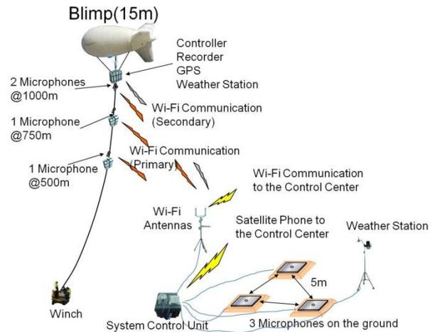
Fig. 4 Boom Measurement System
