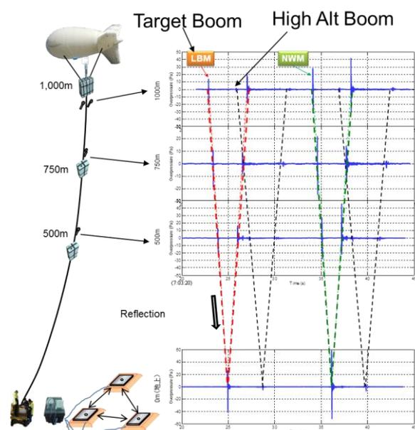
Fig.10 Measured Sonic Booms of No.1
