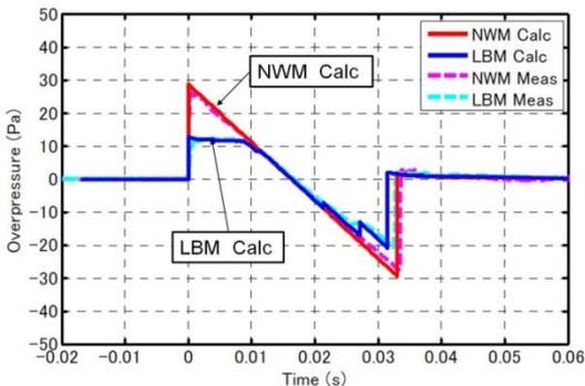
Fig. 12 Sonic Booms at Alt=500m of No.1
