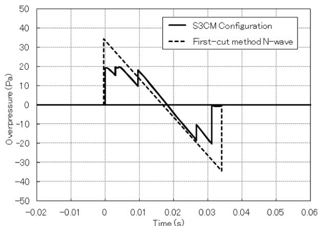
Fig.16 Shaped Sonic Boom Signature of S3CM
