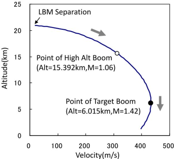
Fig.11 Velocity Profile of LBM
