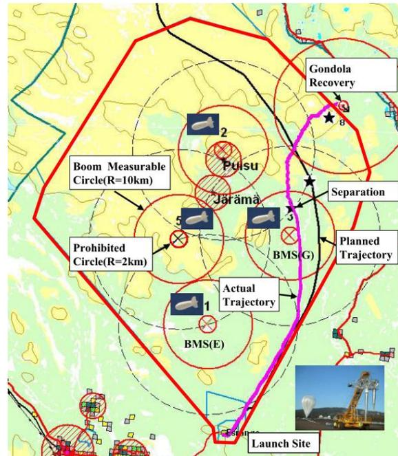
Fig.9 Balloon Trajectory of No.1
