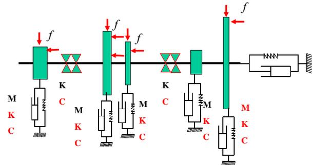
Fig. 2 Rotordynamic fluid forces acting on a rotor.
