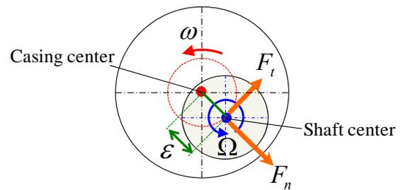
Rotordynamic force effect at  $\omega/\Omega > 0$
