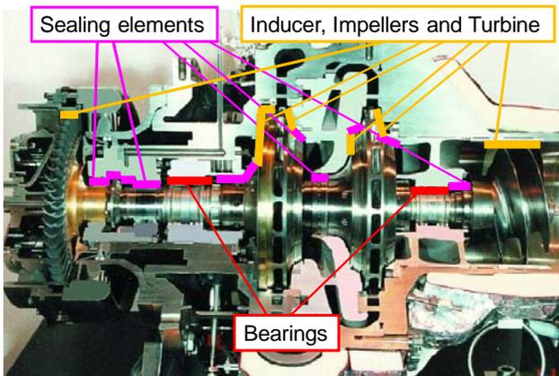
Fig. 1 LE-7 Fuel turbopump
