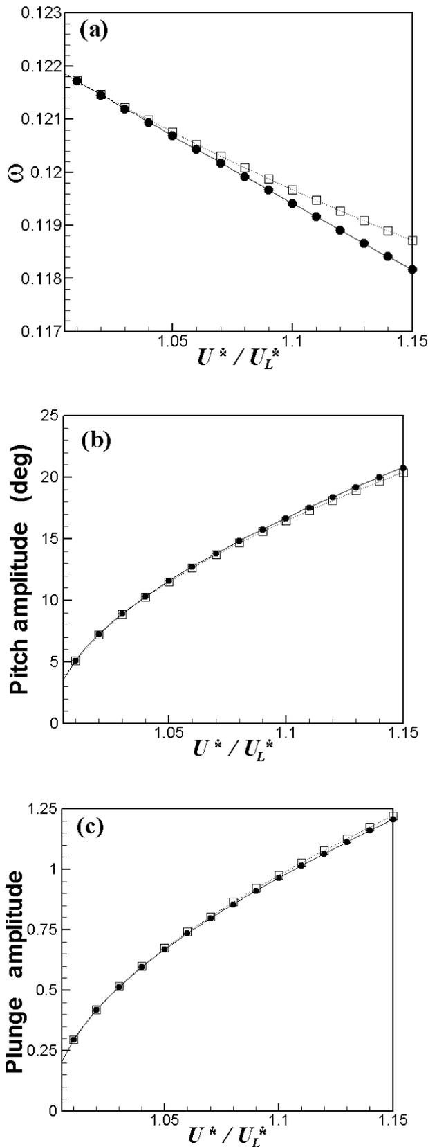
Fig. 3 Wing tip dynamical response: (a) frequency; (b) amplitude of pitch motion; (c) amplitude of plunge motion: —, numerical result; - - - □, HB1; ●, HB3.
