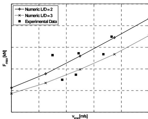
**Fig. 20 : Peak force on 2nd target, 0,65 kg bird surrogates, cylindrical model**
