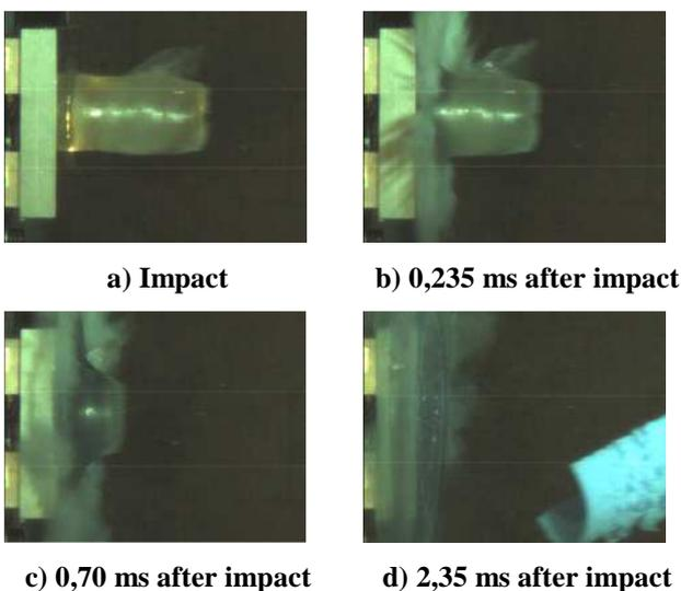
Fig. 4: Impact of a 0,65kg projectile at 124 m/s against the second target
