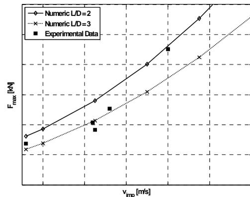
**Fig. 17: Peak force on 1st target, 0,65 kg bird surrogates, cylindrical model**
