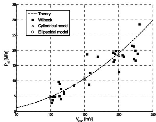
Fig. 10: Stagnation pressure comparison between experimental data and numerical results
