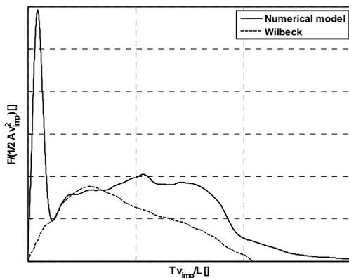
**Fig. 5: Force comparison between cylindrical model and real bird**
