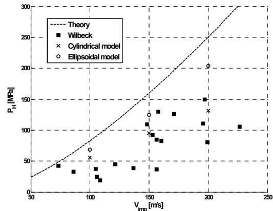
Fig. 9: Hugoniot pressure comparison between experimental data and numerical results
