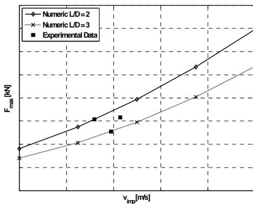
**Fig. 19: Peak force on 2nd target, 1,25 kg bird surrogates, cylindrical model**
