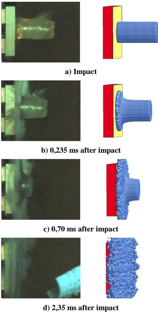
**Fig. 14: Comparison between numerical and experimental deformation, 0,65 kg bird surrogate, speed 124 m/s.**
