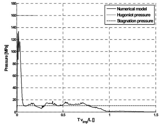
Fig. 8: Comparison between pressure on target of cylindrical model and theoretical results
