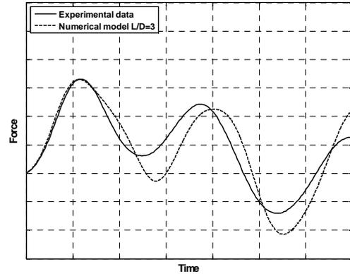
**Fig. 15: Comparison of force on 1st target between experimental data and cylindrical model results, 1,25 kg surrogate, speed 125 m/s, L/D=3**
