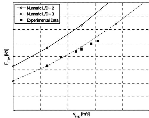
**Fig. 16: Peak force on 1st target, 1,25 kg bird surrogates, cylindrical model**
