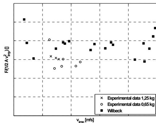
Fig. 6: Non-dimensional peak force on second target
