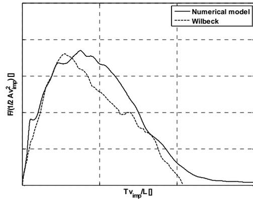
**Fig. 63: Force comparison between ellipsoidal model and real bird**
