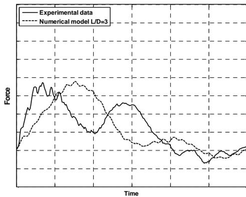
**Fig. 18: Comparison of force on 2nd target between experimental data and elliptical model results, 0,65 kg surrogate, speed 167 m/s, L/D=2.5**
