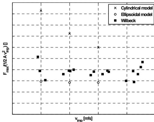
**Fig. 11: Comparison of non-dimensional peak force between Wilbeck data and numerical models results**
