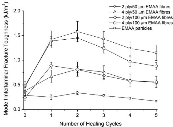
Fig.5. Effect of number of healing cycles on the mode I interlaminar fracture toughness ( $G_{IC}$ ) of the mendable laminates.
