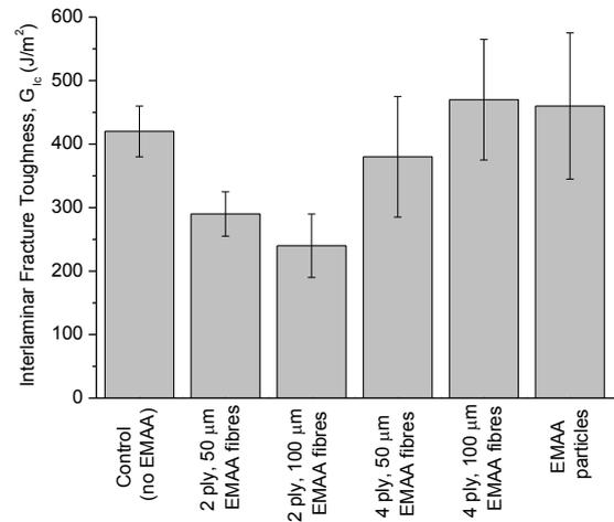
Fig. 1. Mode I critical strain energy release rates ( $G_{Ic}$ ) for the control and mendable EMAA laminates in the original condition.
