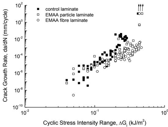
Fig. 7. Fatigue delamination crack growth curves for the unmodified and mendable laminates in the original condition.
