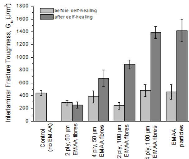
Fig. 2. Mode I interlaminar fracture toughness ( $G_{Ic}$ ) for the control and mendable EMAA laminates in the original condition (before healing) and after self-healing.
