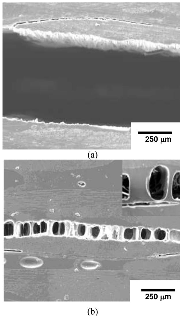
Fig. 4. Scanning electron microscopy images of the delamination crack in a mendable laminate (a) before self-healing and (b) after self-healing. The insert photograph in (b) shows a higher magnification view of the crack bridging ligaments. Note the absence and presence of crack bridging ligaments of EMAA before and after healing, respectively.
