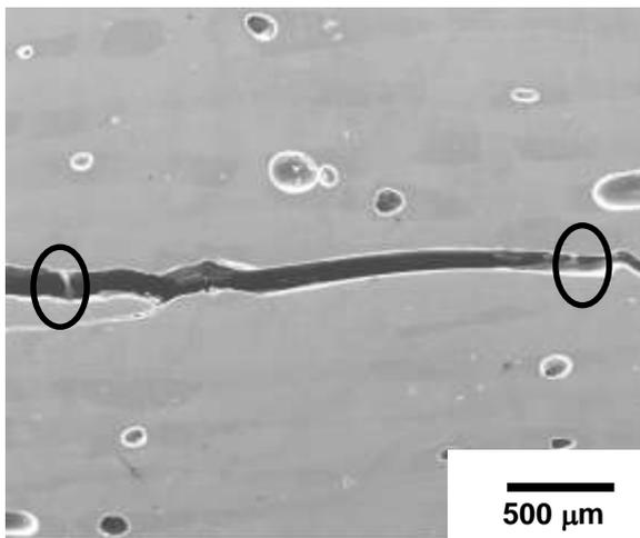
Fig. 5. Cross-section view of the fatigue delamination crack in a mendable laminate. Note the absence of a large-scale bridging traction zone. Only two thin bridging ligaments are visible, which are circled.
