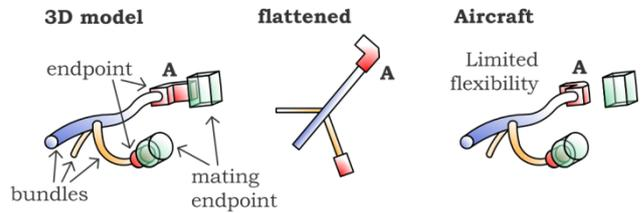
**Fig. 5.** Schematic representation of a 3D wiring harness, the resulting flat representation and the harness during installation. Due to limited bundle flexibility endpoint A may not be able to reach its mating endpoint.
