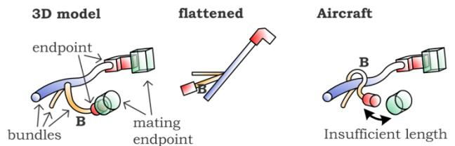
**Fig. 6.** Schematic representation of a 3D wiring harness, the resulting flat representation and the harness during installation. The incorrect orientation of bundle B leads to the situation where there is insufficient length to reach the destination connector.
