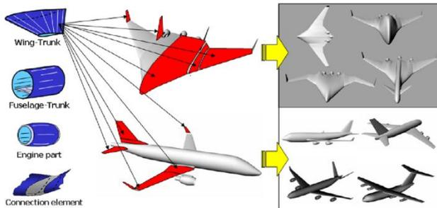
**Fig. 7.** Generation of different aircraft configurations and variants using the HLP modeling approach [8]
