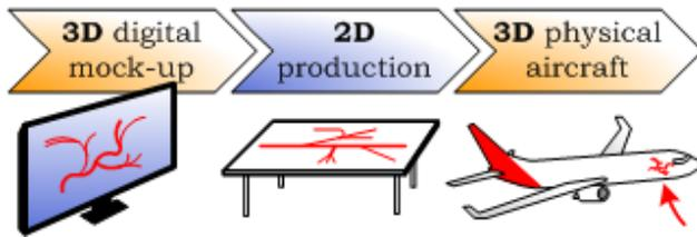
**Fig. 2.** The wiring harness is designed in 3D, produced on a flat table and installed in 3D.
