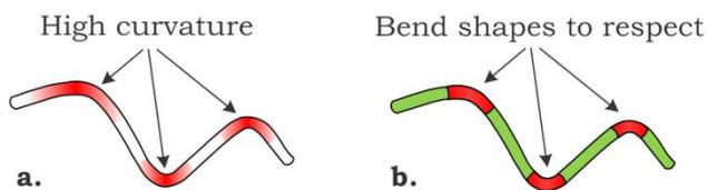
**Fig. 10.** The curvature of wiring harness bundles is analyzed (a) and sections with bend radii violating bending rules are identified (b).
