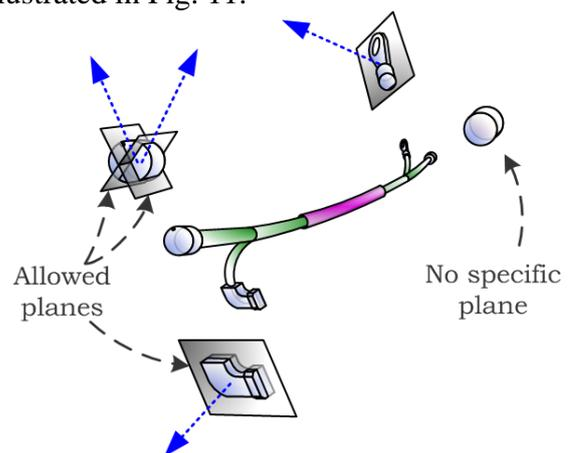
**Fig. 11.** For each endpoint component, the allowed flattening plane(s) are determined based on component specific rules.
