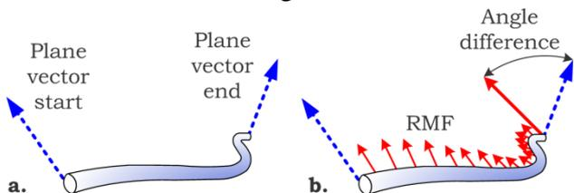
**Fig. 13.** The plane vectors at each end of a bundle are computed (a) and the effective angle difference between both planes is computed (b).
