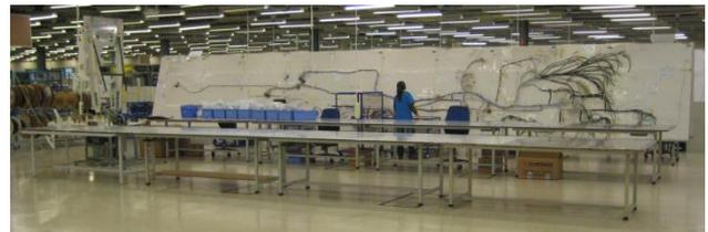
**Fig. 1.** A wiring harness on a formboard. Source: Fokker Elmo B.V.
