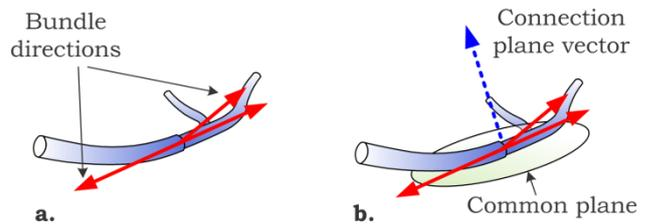
**Fig. 9.** At a bundle connection point, direction vectors are determined (a) and the closest common plane is computed (b).
