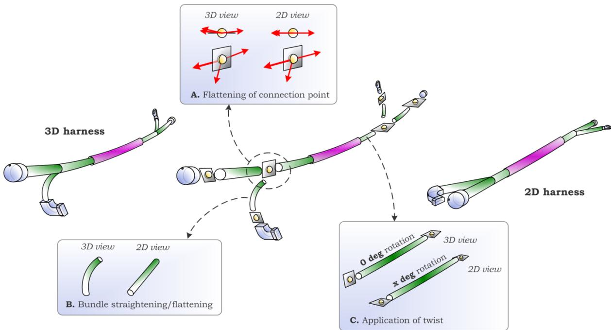
**Fig. 12.** Schematic illustration of the procedure to generate a 2D wiring harness representation. Each connection point HLP is flattened (A), each bundle HLP is flattened (B) and a twist angle is applied to each bundle (C).
