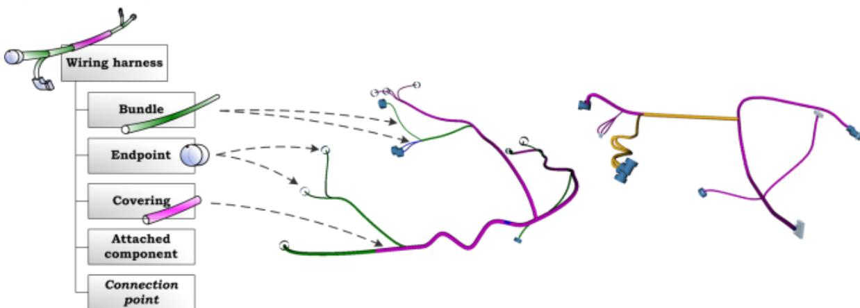
**Fig. 8.** Left: Breakdown of wiring harness components. Center and right: Two 3D wiring harness models composed of instances of the wiring harness HLPs
