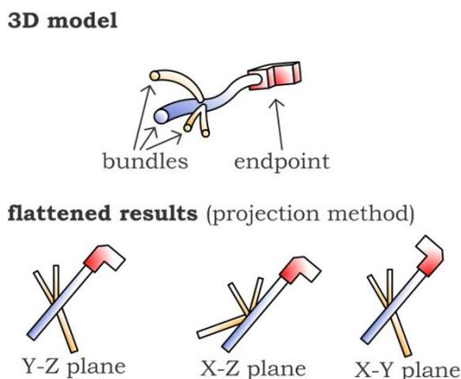
**Fig. 4.** Schematic representation of a 3D wiring harness and resulting flat representations, depending on the projection plane.
