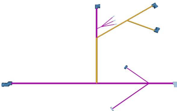
**Fig. 17.** Example 2: 2D representation of the wiring harness shown in the right part of Fig. 8.
