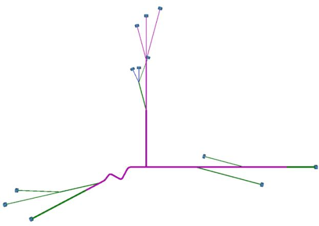
**Fig. 16.** Example 1: 2D representation of the wiring harness shown in the center of Fig. 8.
