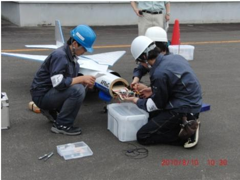
Fig. 14. Preflight check on onboard avionics.
