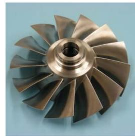
Fig. 11. The fabricated first-stage fan in the prototype counter-rotating axial fan turbojet engine.
