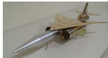
Fig. 3. The modified configuration M2006prototype for constructing a prototype vehicle.
