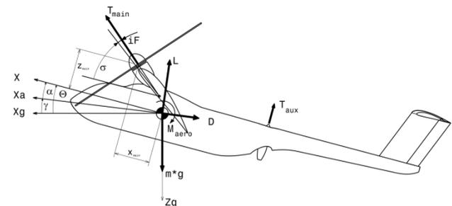
Fig. 5. Forces and moments in longitudinal motion
