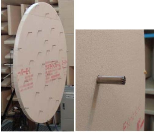
Fig. 6. Microphone array and microphone installation
