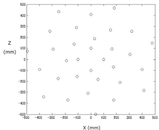
Fig. 5. Multi-arm-spiral microphone arrangement
