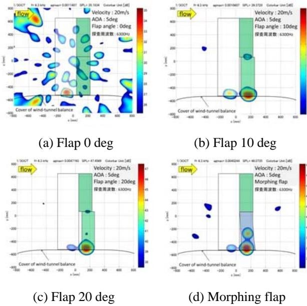
Fig.16.  $U=20\text{m/s}$ ,  $\alpha=5\text{ deg}$ ,  $f=6300\text{Hz}$
