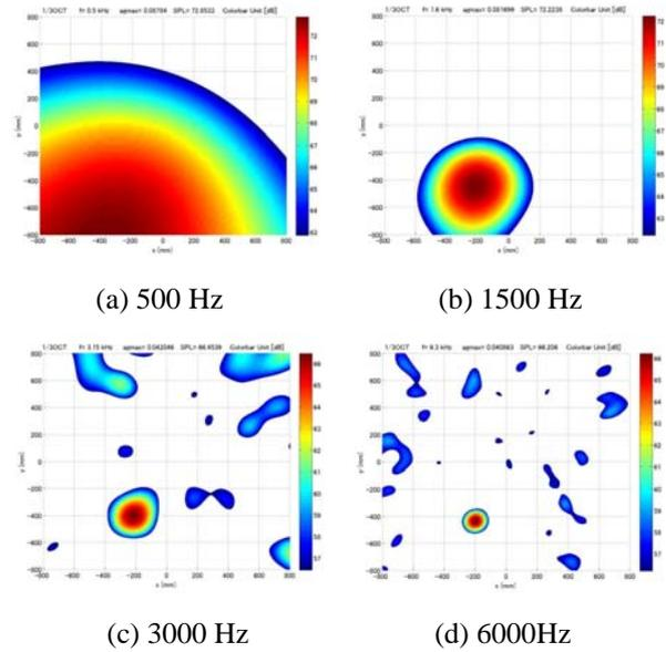
Fig. 8. Noise source survey for speaker test
