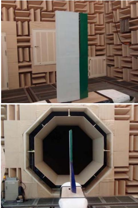
Fig. 4. Model installation in wind tunnel test section
