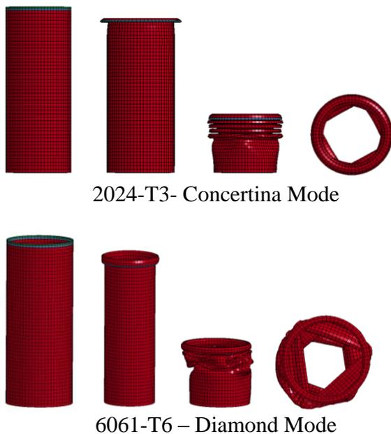
**Fig. 4. Crushing modes of aluminium tube.**
