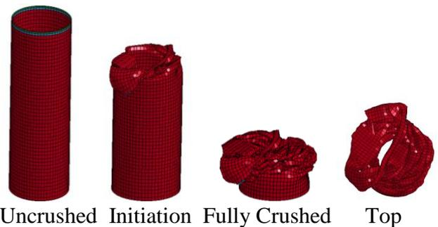
**Fig. 8.- Crushing mode of CFRP**
