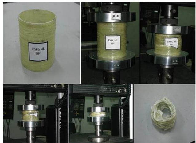
**Fig. 7.- Experimental crushing of glass/epoxy.**
