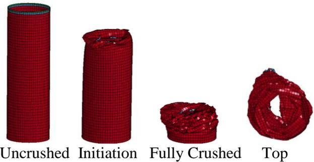
**Fig. 6. Crushing mode of GFRP.**
