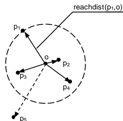
**Fig. 5.** Remoteness evaluation in the Local Outlier Factor (LOF) algorithm [9] to determine outliers for the capacity curve generation. Graphical illustration of the reach dist determination for an exemplary case of  $N = 4$  nearest neighbors.
