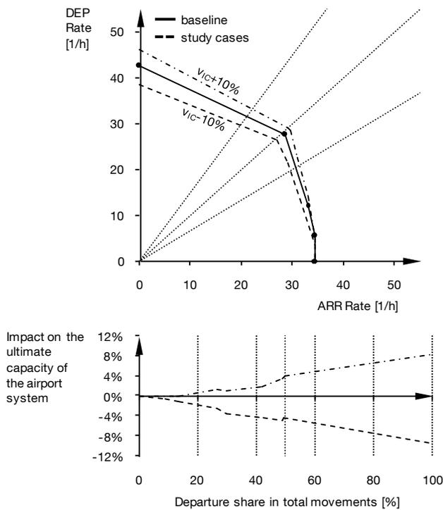
**Fig. 8.** Representation of the ultimate airport capacity impact of medium jet aircraft operations with increased/decreased initial climb speeds ( $v_{IC}$ ) compared with a baseline case.
