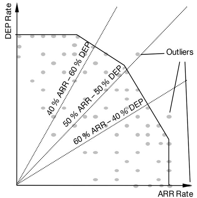
**Fig. 2.** Capacity curve representation based on E. Gilbo [1] to visualize the capacity of an airport system for various arrival to departure ratios.
