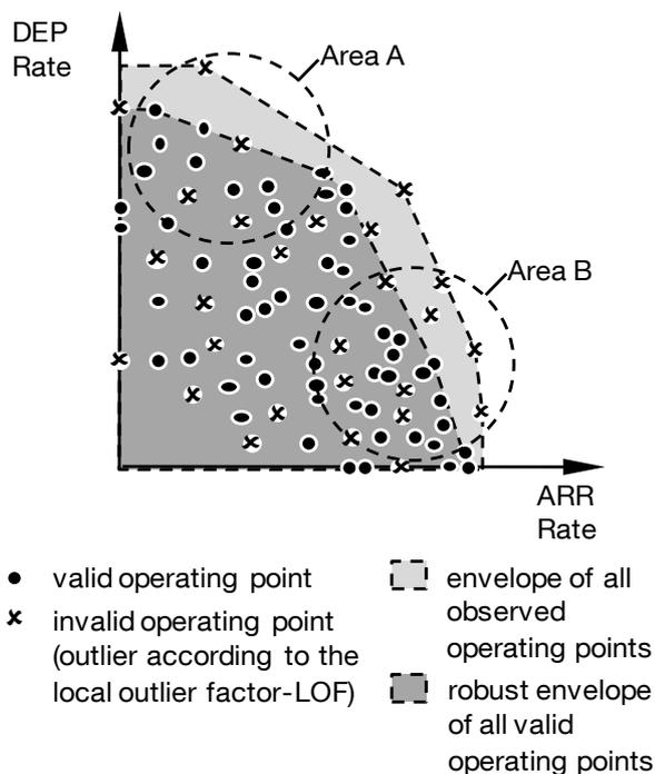
**Fig. 4.** Example application of the local outlier factor [9] as rejection criterion in the context of the generation of capacity curves.
