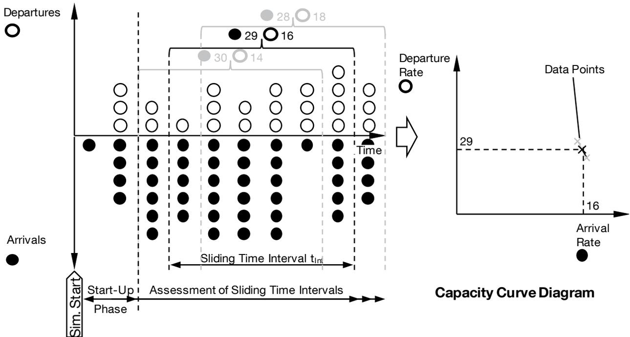
**Fig. 3.** Basic data generation using sliding time intervals.
