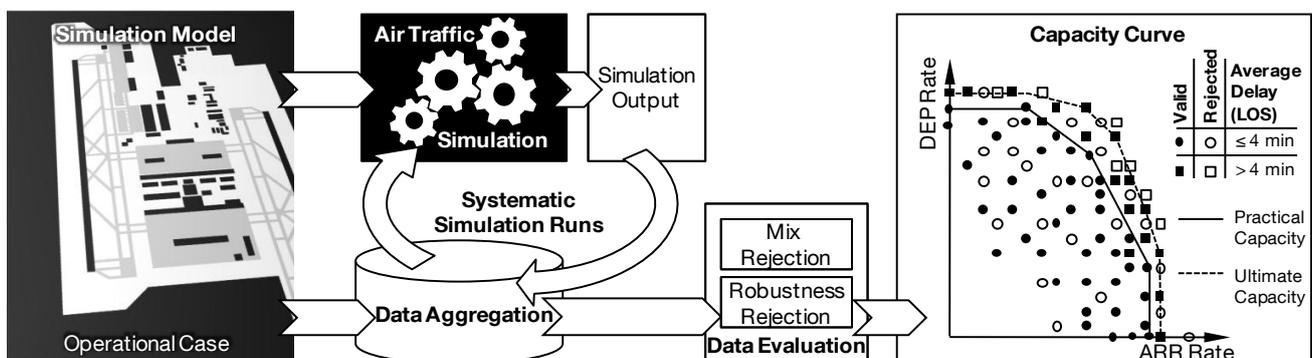
**Fig. 1.** Overview of the technical approach to generate capacity curve diagrams visualizing the operational limitations of an airport system for a predefined operational case based on air traffic data generated by fast-time simulations.
