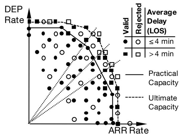
**Fig. 6.** Resulting capacity curve diagram for both, practical and ultimate capacity envelopes of a given simulated airport system.
