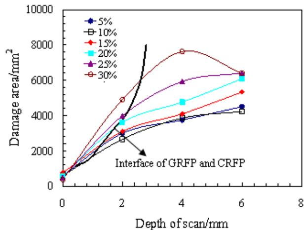
Fig. 7 Relations of proportion of front face, resin crack length and damage area of post-impacted composite laminates
