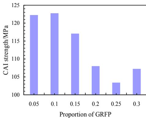
Fig.9 Relations between proportion of front face and compression after impact (CAI) strength
