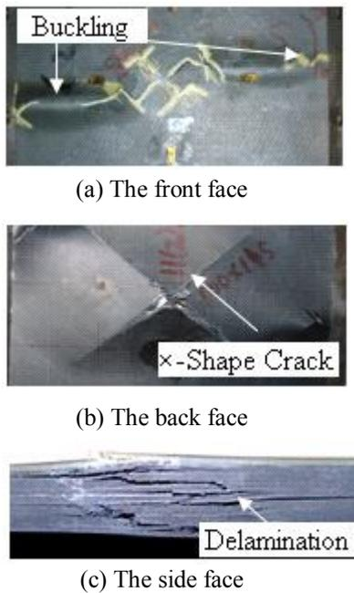
Fig.8 Damage of impacted composite laminate when failed
