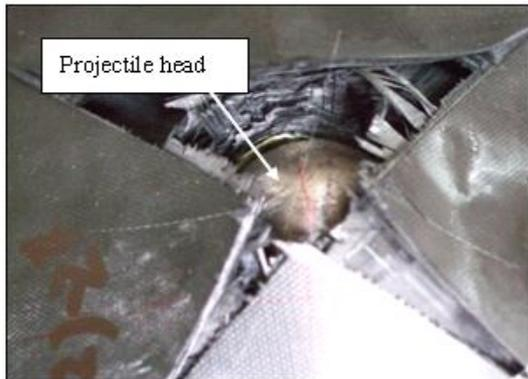
Fig. 4 Damage of CRFP
