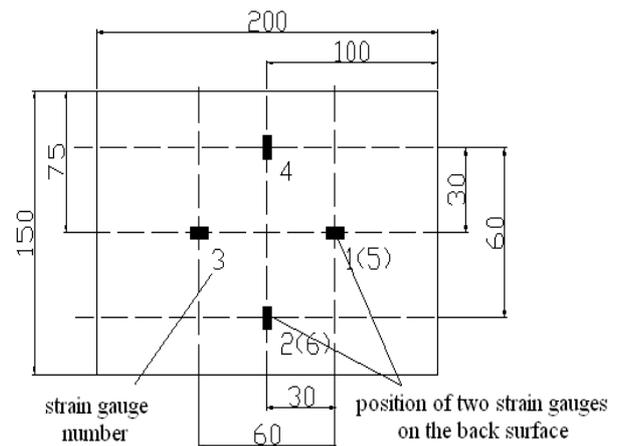
Fig. 2(b) Position of strain gauge
