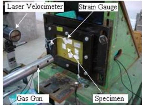
Fig. 2(a) Picture of Impact test fixture
