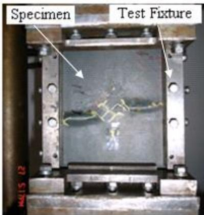
Fig. 3 The post-impact compression test rig
