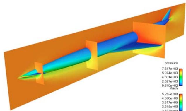
Fig. 3. Mach 5 CFD results from Argo<sup>®</sup>.
