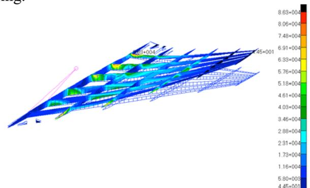
Fig. 6. Wing deflection at 2.5g at Mach 5, colored by stress level.
