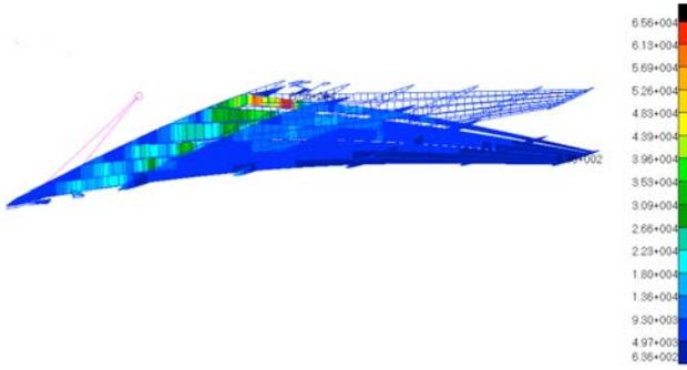
Fig. 6. Wing deflection at -1g at Mach 5, colored by stress level.
