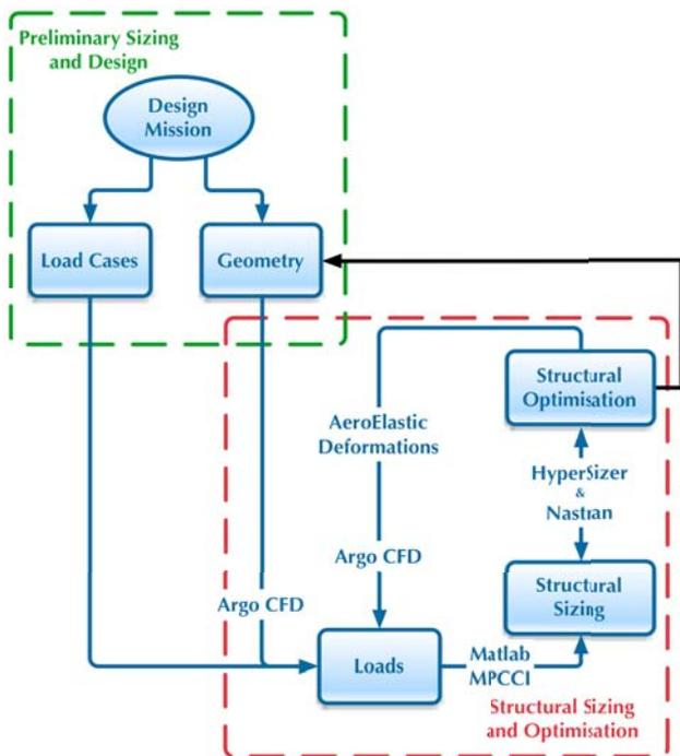
Fig. 2. The Sizing Process Used in the Optimisation of the A2 Structure.
