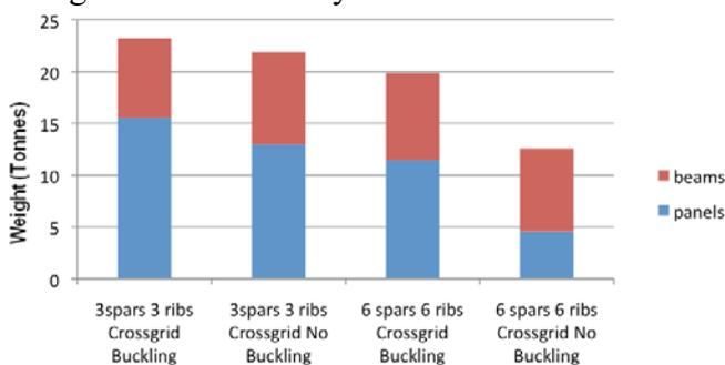
Fig. 7. Influence of buckling on wing weight.
