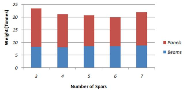
Fig. 5. Wing weight with 6 ribs.
