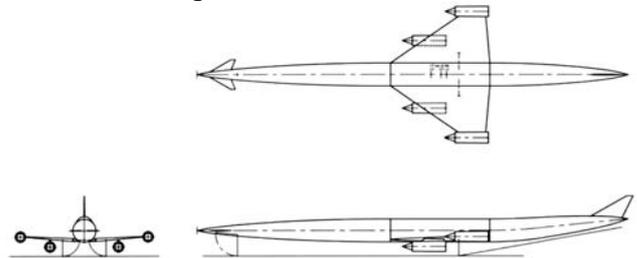
Fig. 1. The LAPCAT A2 Configuration.
