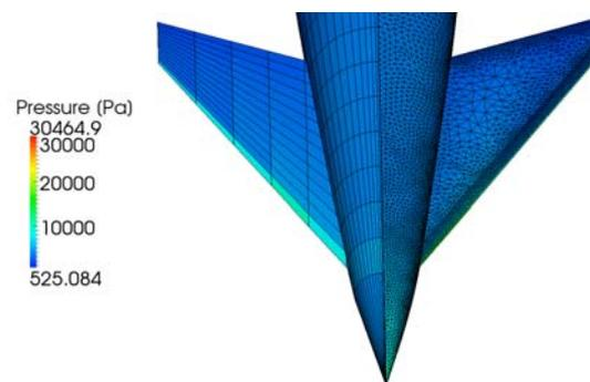
Fig. 4. FE/CFD mesh interpolation.
