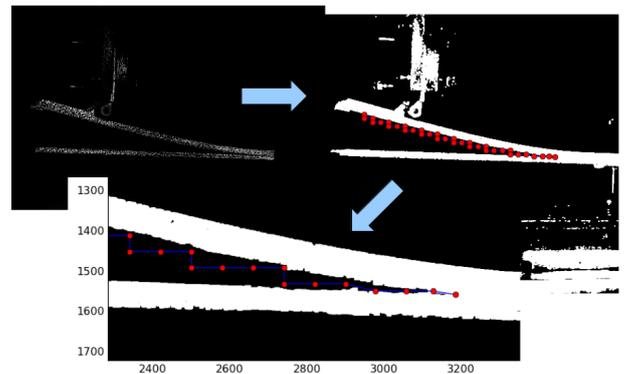
**Fig. 10** Image processing to find the delamination front
