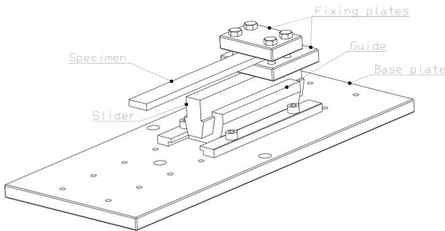
**Fig. 8** FRMM loading fixture
