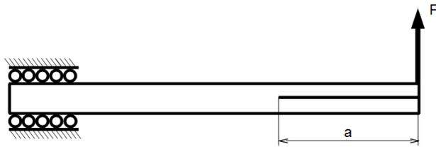
**Fig. 2** Fixed ratio mixed mode test
