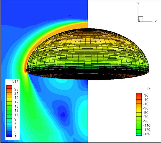
Fig. 5 Pressure on the body surface
