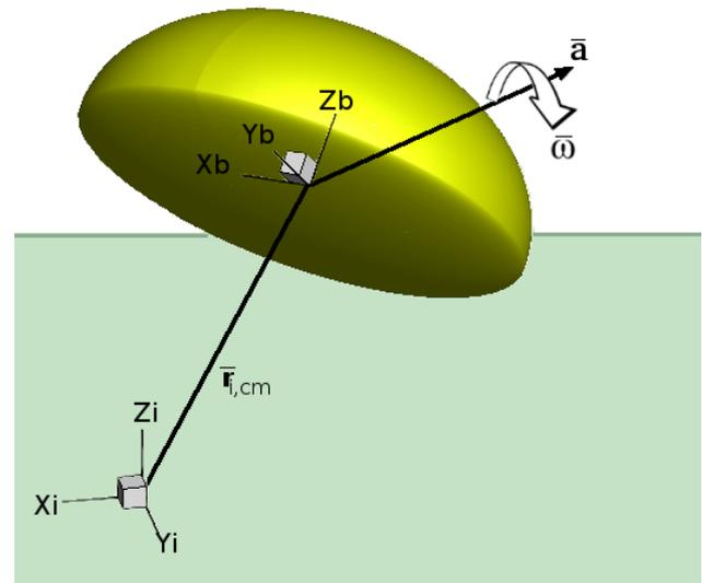
**Fig. 4** Two coordinate systems used to express the unconstrained motion of a rigid body
