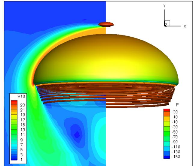
**Fig. 8** Iso-surface of  $Q$  coloured by pressure
