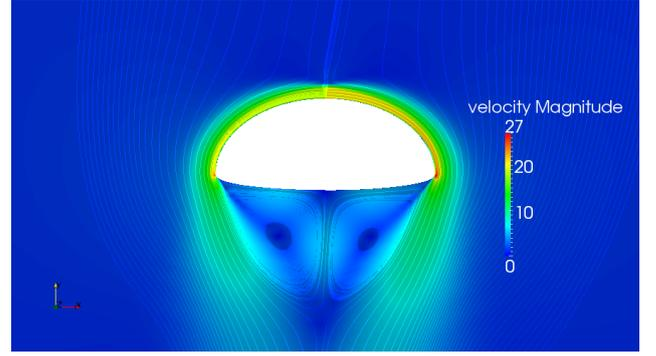
Fig. 6 Asymmetric Coanda effect - velocity magnitude and streamlines
