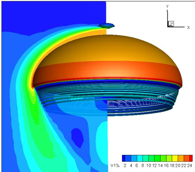
**Fig. 7** Iso-surface of  $Q$  coloured by velocity magnitude
