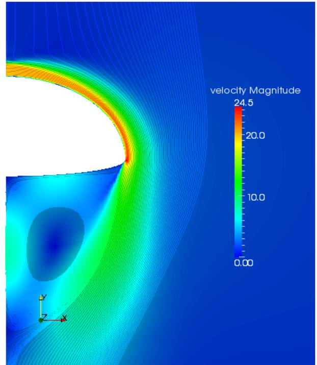
**Fig. 3** Symmetric Coanda effect - flow picture, only one half is shown
