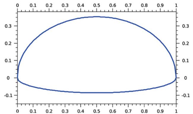
Fig. 1 Cross section of the Coanda effect UAV
