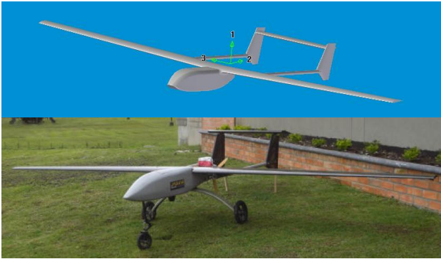
Fig. 6. UPB's CAD render (above) and TELSAT prototype (below) of Jaguar UAS.
