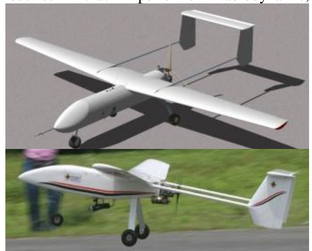
Fig. 8. AURA CAD model (above), AURA JR (Below).
