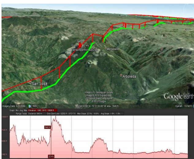
Fig. 12. Analysis of a low altitude observation flight by using Google Earth and MATLAB. The vertical terrain contour reaches altitudes from 500ft until 10,000 ft.
