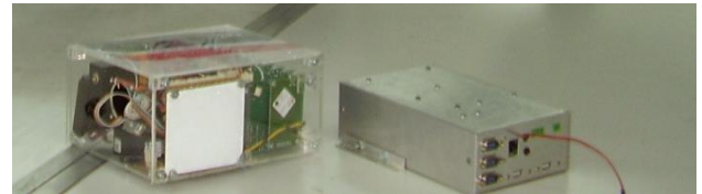
Fig. 7. AURA's sensors (left) and flight computer (right).
