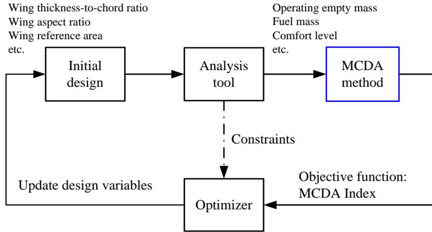
Fig. 1 The Framework of Incorporating MCDA Techniques in Aircraft Design
