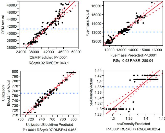
**Fig. 6** The Actual by Predicted Plots of OEM, Fuel Mass, Utilization/(Block time), and Passenger Density, when using SAW Index as an Objective Function
