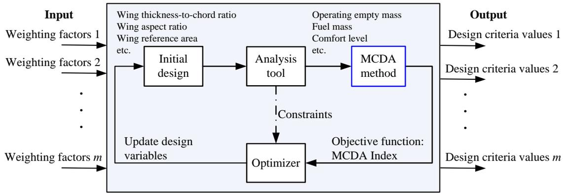
**Fig. 4** The Overview of Surrogate Modeling Process for Design Criteria in Terms of Weighting Factors
