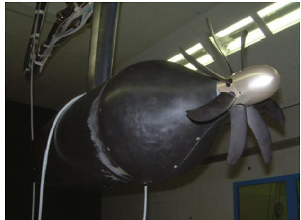
Fig. 13. Minimum body wind tunnel test
