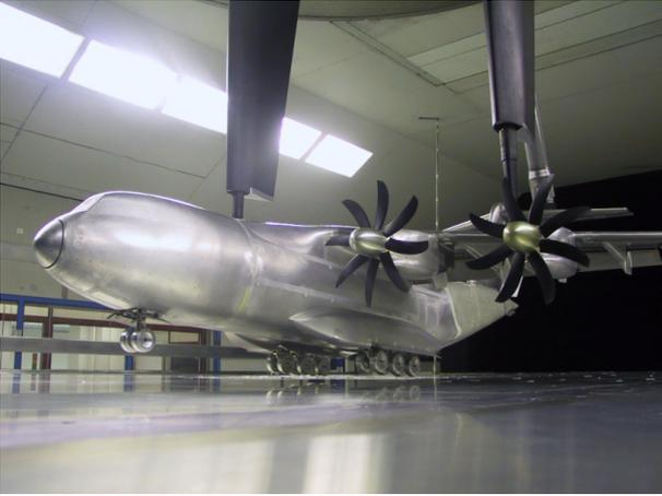
Fig 9. Installed propeller test
