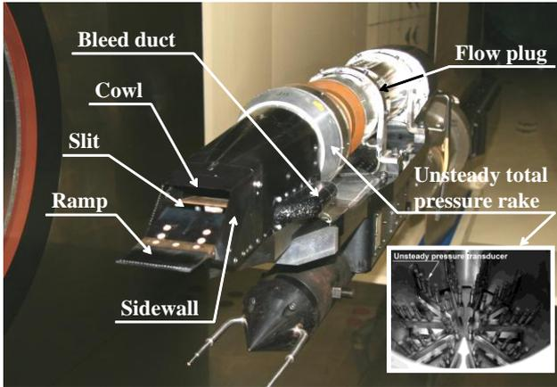
Fig.7 Experimental model
