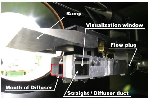
Fig.2. Simplified inlet model
