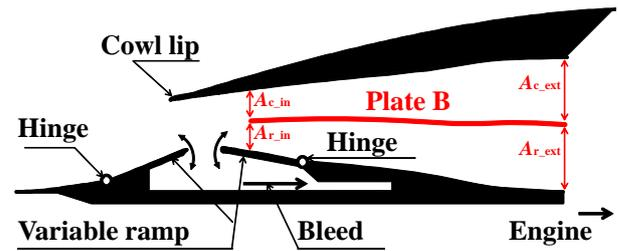
(b) Configuration of splitter plate B
