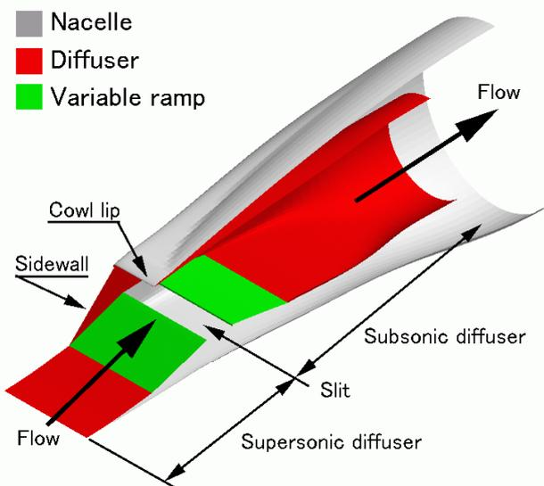
Fig.5 Supersonic inlet with variable ramp
