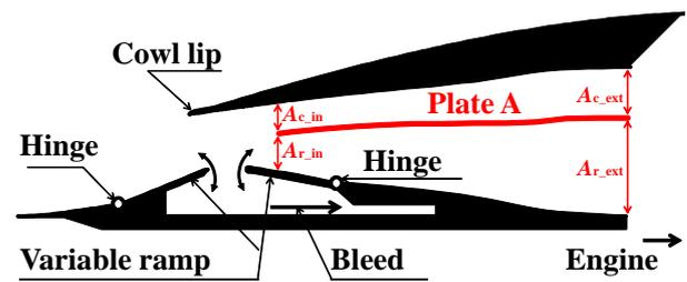
(a) Configuration of splitter plate A
