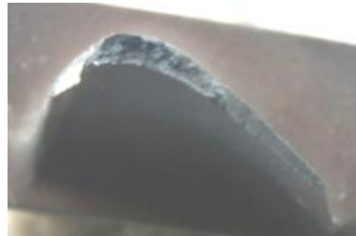
Fig.3 Macro feature of fracture surface of SC blade by creep
