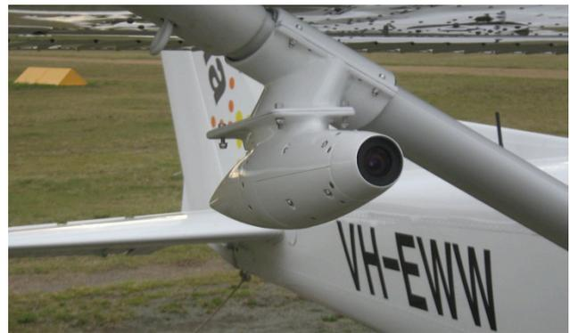
Fig. 2. Detect-and-Avoid EO sensor fitted to the wing strut of the ARCAA Airborne Systems Laboratory
