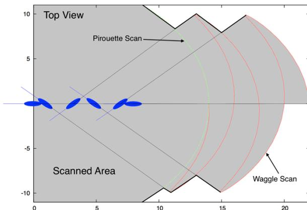
Fig. 3. Area scanned by the laser in the pirouette and waggle flight modes
