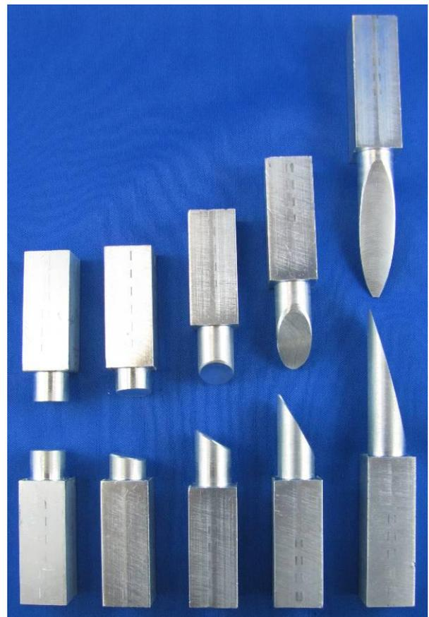
Fig. 2: Tensile butt-joints with 0°, 15°, 30°, 60° and 75° bonding angles (from left to right)
