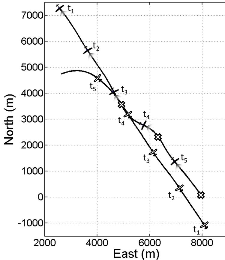
**Fig. 6** Aircraft flight paths (solid lines) during a head-on collision avoidance experiment (overhead view). The host Cessna and target aircraft positions are indicated by the dark and light aeroplane markers, respectively. The crosses ( $\times$ ) mark the locations of avoidance waypoints issued by the sense-and-avoid system.
