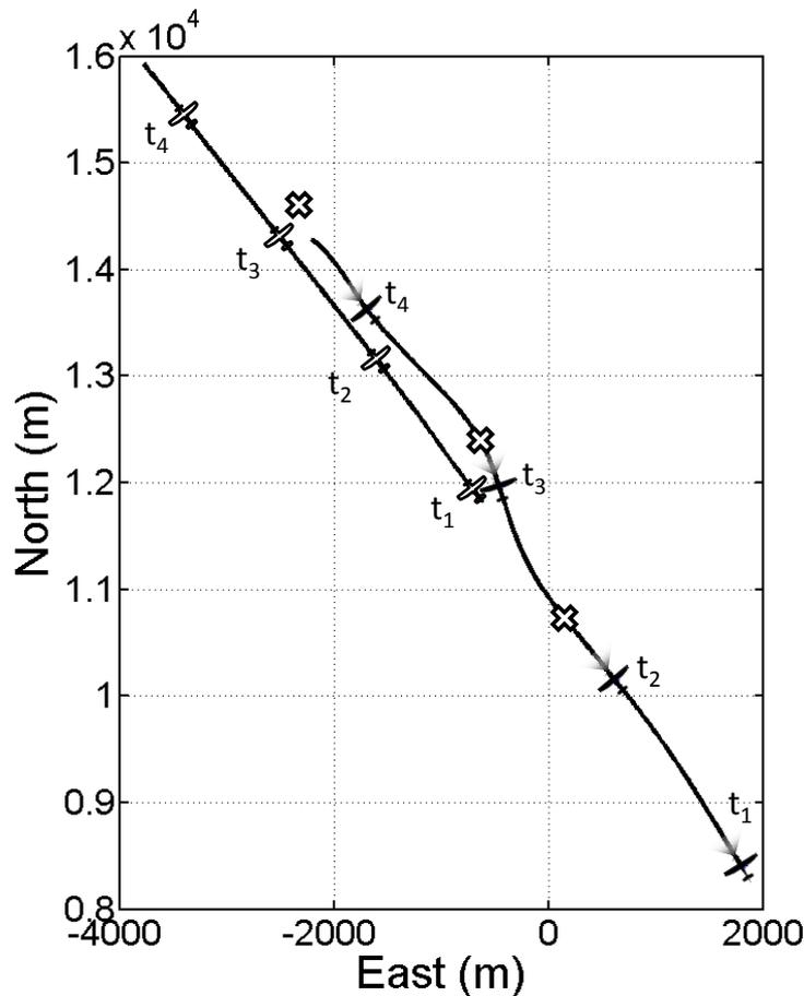
**Fig. 5** Aircraft flight paths (solid lines) during a tail-chase collision avoidance experiment (overhead view). The host Cessna and target aircraft positions are indicated by the dark and light aeroplane markers, respectively. The crosses ( $\times$ ) mark the locations of avoidance waypoints issued by the sense-and-avoid system.
