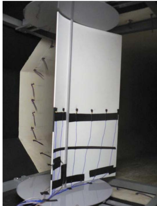
**Fig. 7** The rotational point of the wing is at the spar which is placed closer to the leading edge than the trailing edge.
