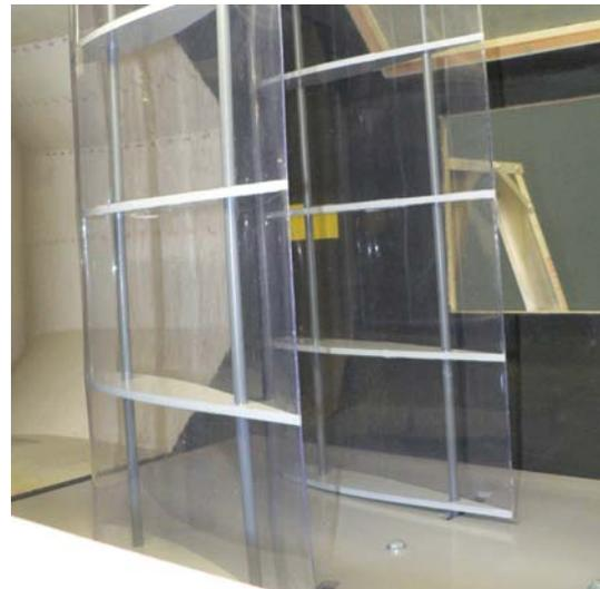
**Fig. 5** Gust generating wings are slotted into the blocking boards and their controlling rods pass through the slots at the bottom of the tunnel.
