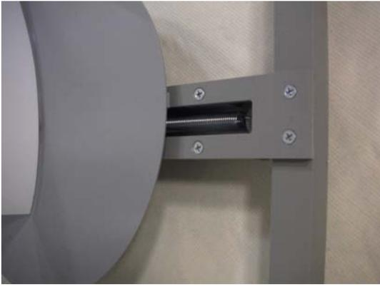
**Fig. 3** The translational springs are limited in their direction of movement by the rail system.
