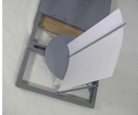
**Fig. 6** The test wings slot into the end plates.
