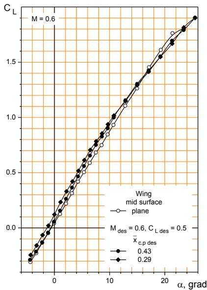
Fig. 7. The effect of design position of the wing section center of pressure line on the model lift coefficient
