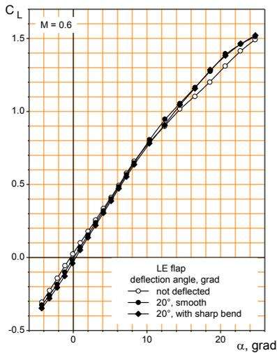
Fig. 11. The effect of wing leading edge flap junction smoothness on the model lift coefficient
