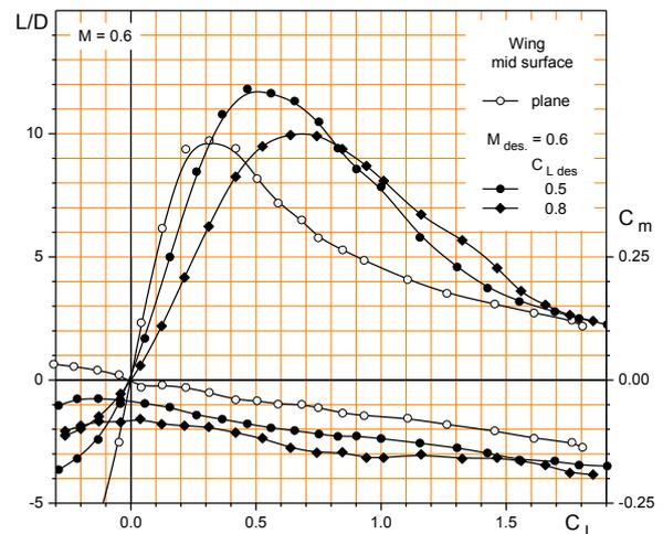
Fig. 6. The effect of all wing mid surface deformation on the model lift-to-drag ratio and the pitching moment coefficient
