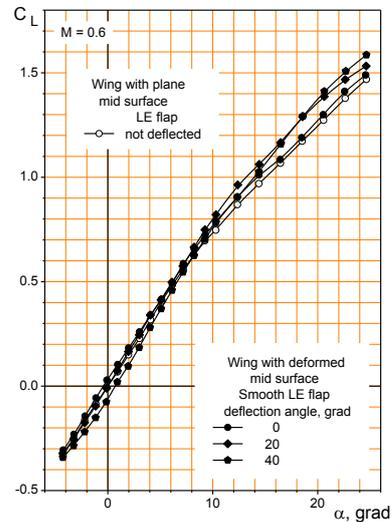
Fig. 9. The effect of wing leading edge flap smooth deflection on the model lift coefficient
