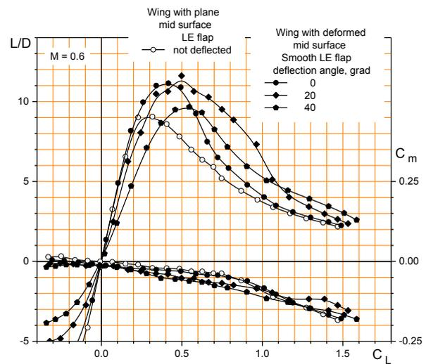
Fig. 10. The effect of the wing leading edge flap smooth deflection on the model lift-to-drag ratio and the pitching moment coefficient
