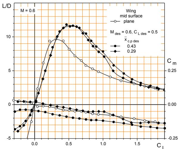
Fig. 8. The effect of design position of the wing section center of pressure line on the model lift-to-drag ratio and the pitching moment coefficient
