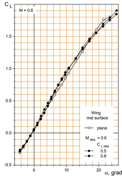
Fig. 5. The effect of all wing mid surface deformation on the model lift coefficient
