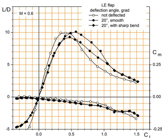
Fig. 12. The effect of wing leading edge flap junction smoothness on the model lift-to-drag ratio and the pitching moment coefficient
