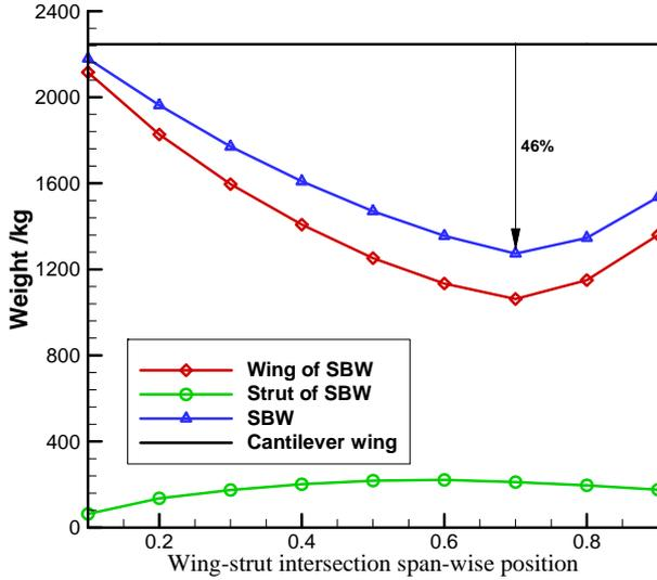
Fig. 5. Weight reduction for different wing-strut intersection
