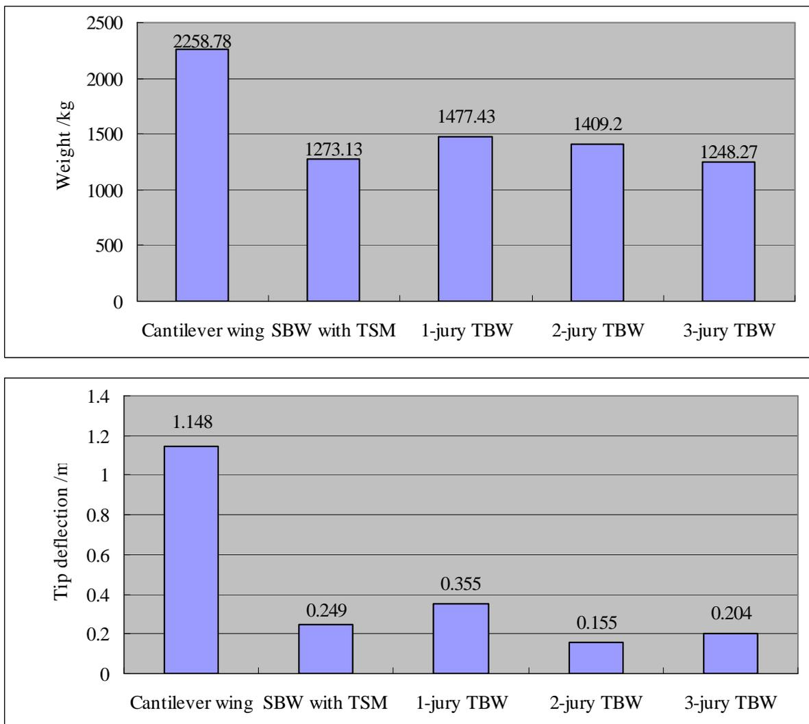
Fig. 10. Comparison of different TBW configurations with cantilever wing
