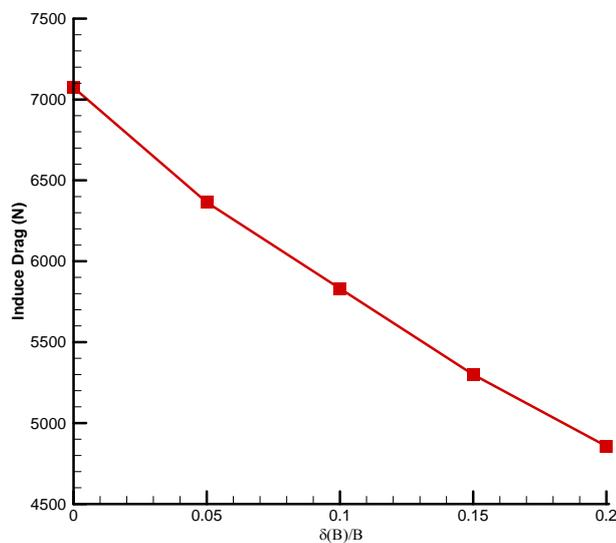
Fig. 12. Effect of span on induced drag
