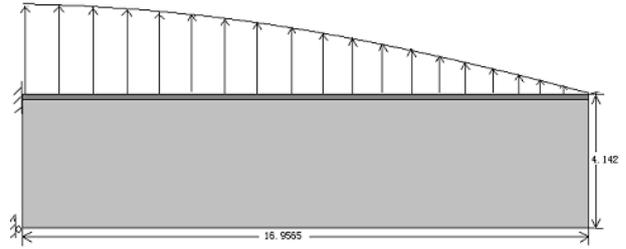
Fig. 6. TBW ground-structure, boundary conditions and loading
