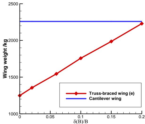
Fig. 11. Effect of span on weight of TBW
