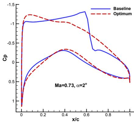
a) Comparison of the pressure coefficient distributions of the optimized and baseline airfoils
