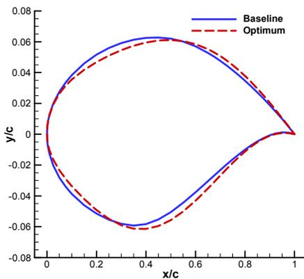
b) Comparison of the geometries of optimized and baseline airfoils
