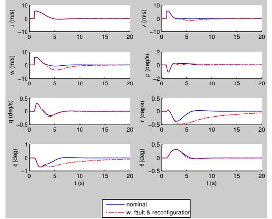
**Fig. 4** Evolution of helicopter states: nominal and after fault & reconfiguration
