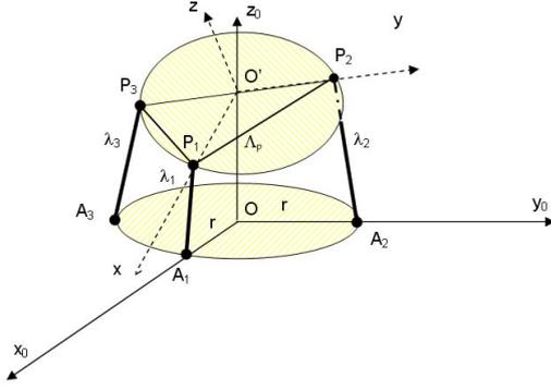
**Fig. 1** Geometric configuration of a swashplate and actuators mechanism
