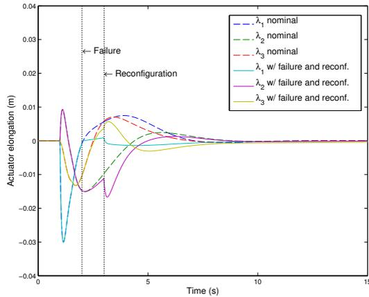
**Fig. 5** Evolution of actuators lengths: nominal and after fault & reconfiguration
