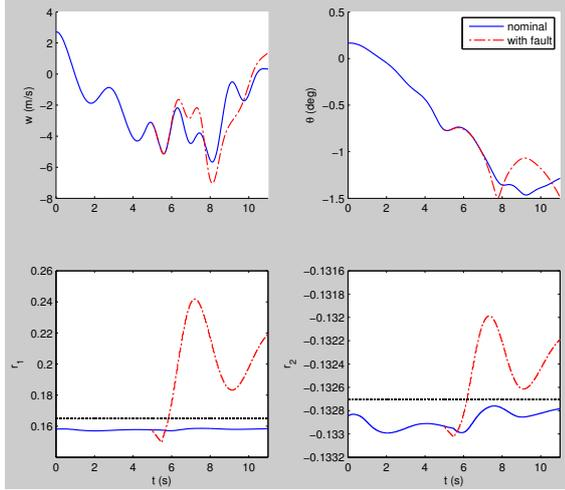
**Fig. 2** Evolution of helicopter dynamics and residual components in presence of actuator failure
