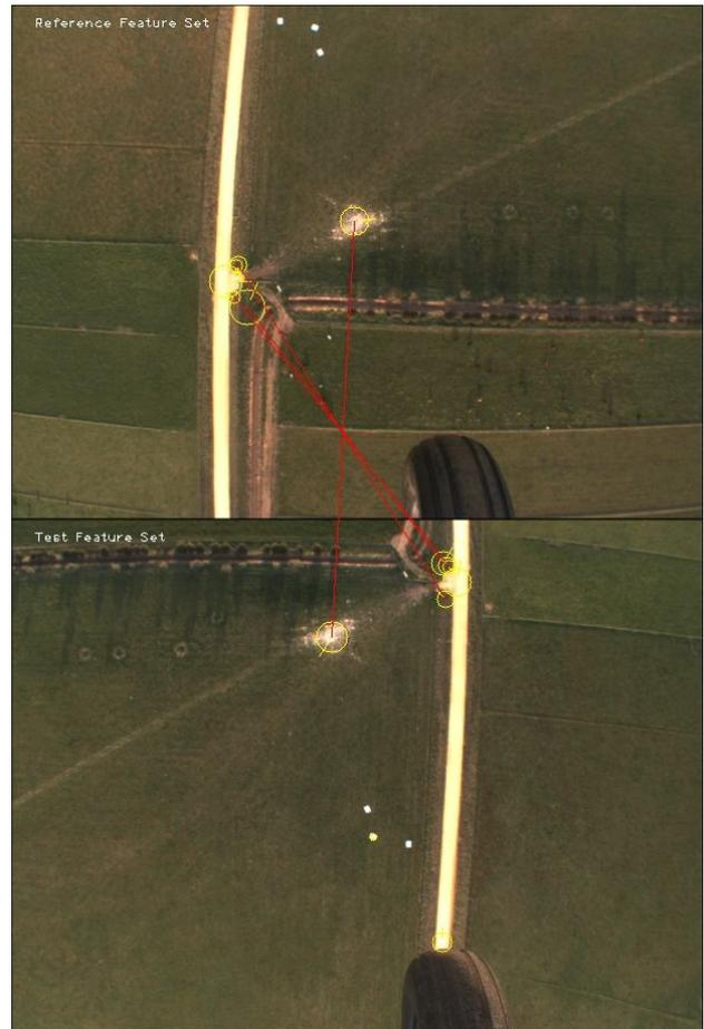
FIG. 5. EXAMPLE OF SURF FEATURE DETECTION AND MATCHING.
