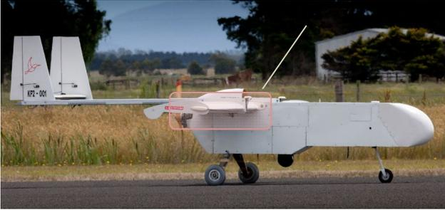
FIG. 2. AIR DATA PROBE ON KINGFISHER 2 UAV.
