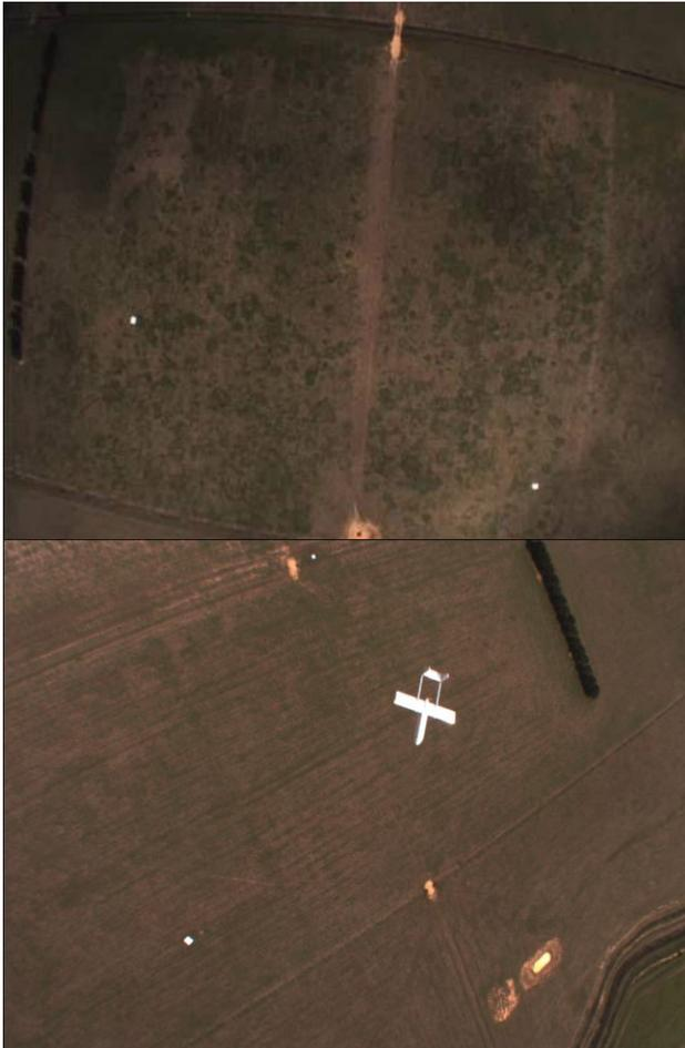
FIG. 4. EXAMPLE OF WHITE TARGETS USED IN FURI CTD FOR SLAM FEATURES.
