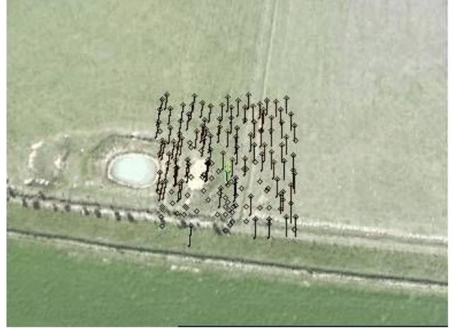
FIG. 3. EXAMPLE OF OPTICAL FLOW VECTORS IN REGION AROUND CENTER OF FRAME.
