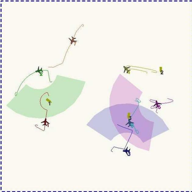
Figure 1(a): Simulated scenario at time 102 seconds. UAV 3 (blue) was tracking target 3 in cooperation with UAV 5 (purple). The fused track on target 3 was accurate enough for UAV 6 (cyan) to carry out attack. UAV 2 (green) was tracking target 1 and waiting for assistance from UAV 1 (red) and 7 (orange).
