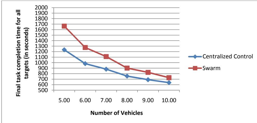
Figure 1: Comparison of swarm control and centralized control.
