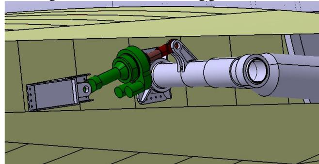
Fig.9. EMA installation-landing gear retracted
