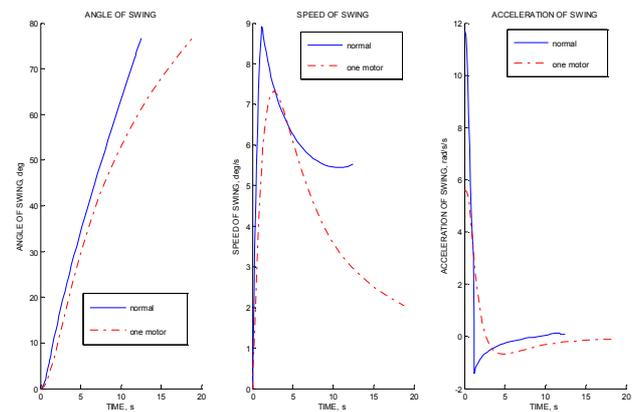
Fig.5. EMA landing gear swing dynamics
