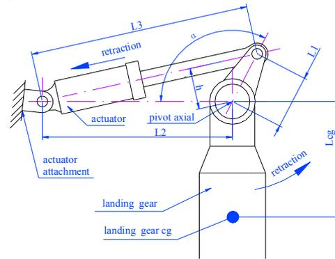
Fig.3. Landing gear kinematics
