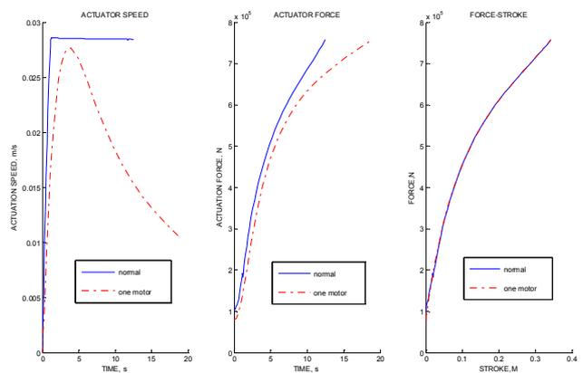
Fig.6. EMA actuator dynamics
