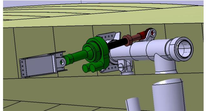
Fig.8. EMA installation-landing gear lowered
