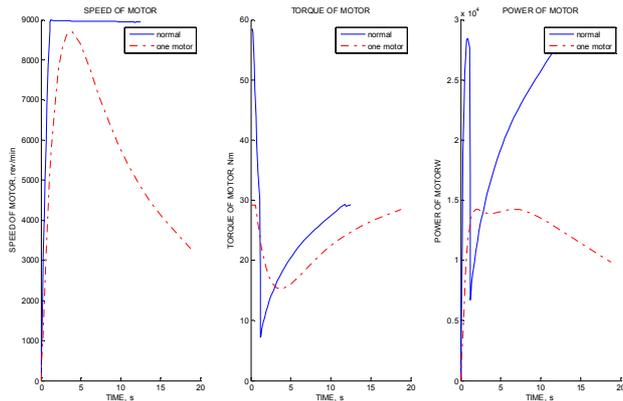
Fig.7. EMA motor dynamics
