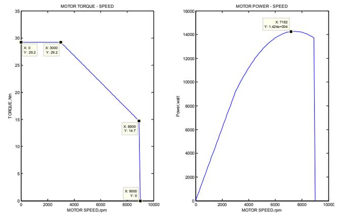
Fig.4. EMA Motor speed-torque and speed-power curves
