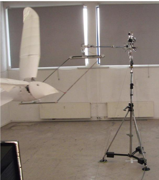
**Fig. 3.** An earlier model flying in the test stand RL3.
