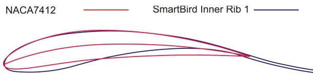
**Fig. 12.** SmartBird's wing section and the section NACA7412 applied during the design process.
