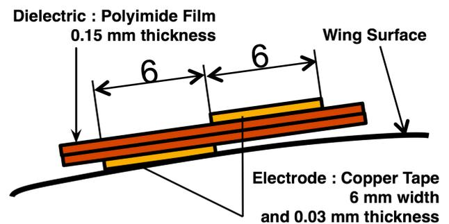
**Fig. 5** Geometry of DBD plasma actuator on the main wing
