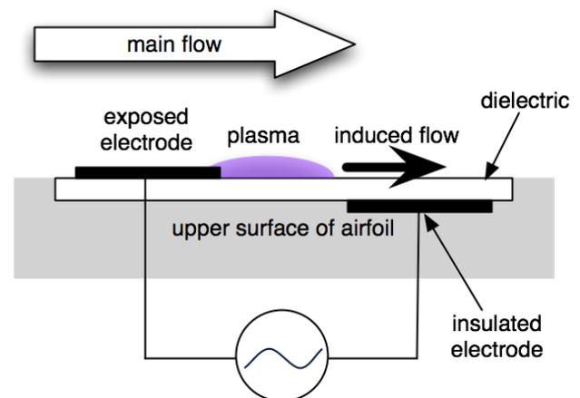
**Fig. 1** SDBD plasma actuator placed in the direction following to the main flow
