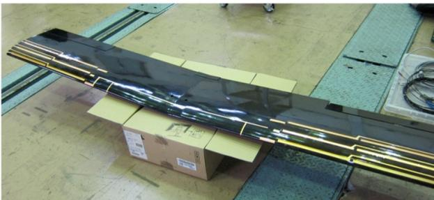
**Fig. 3** DBD plasma actuator on the main wing
