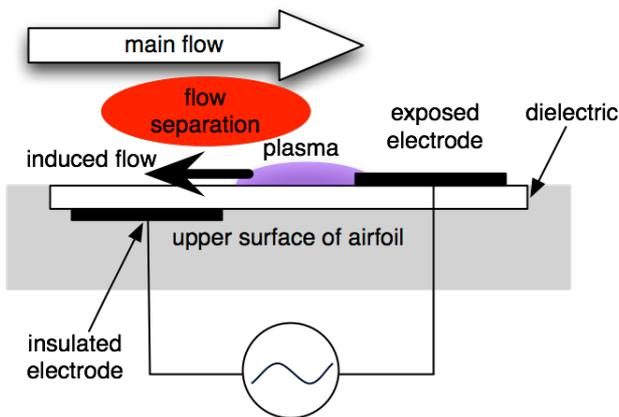
**Fig. 2** SDBD plasma actuator placed in the direction facing to the main flow
