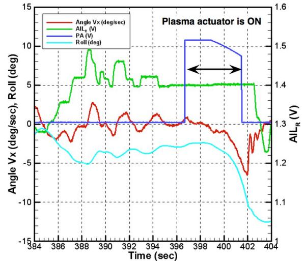
**Fig. 7 Time history of the roll angle (cyan), the roll angle velocity (red), the aileron angle (green), and the signal for plasma actuator (blue)**
