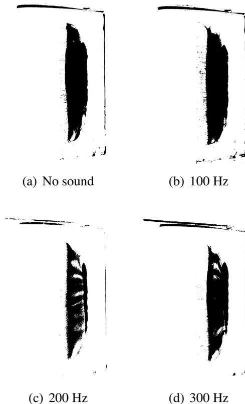
**Fig. 9** Processed images of the wind tunnel results in the KH amplification range
