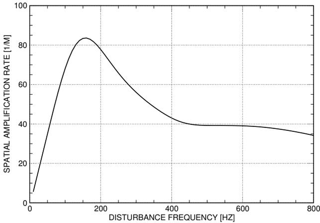
Fig. 5 KH spatial amplification for  $x/c = 0.60$
