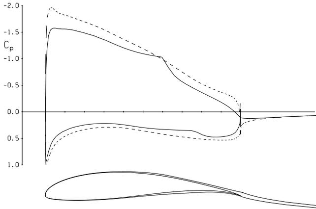
**Fig. 2** Pressure distribution for  $\alpha = 4^\circ$
