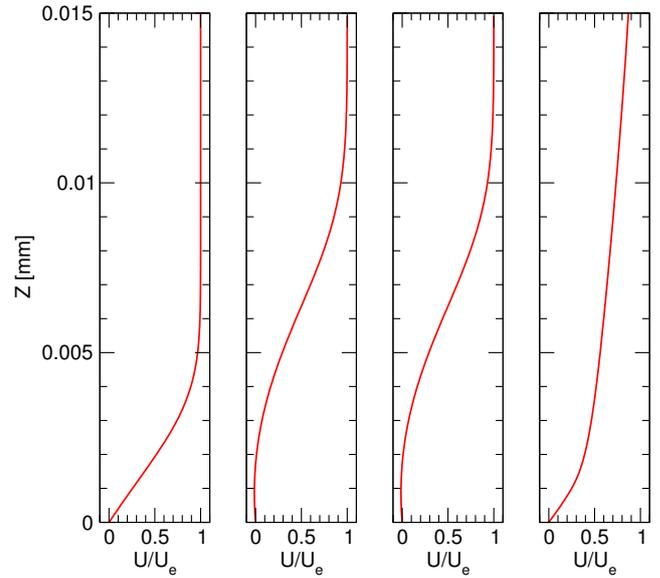
**Fig. 3** Boundary layer velocity profiles used for the linear stability computations
