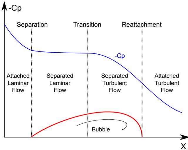
**Fig. 1** Typical flow structure in a laminar separation bubble
