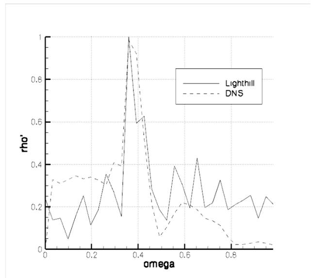
**Fig. 15** Comparison between Lighthill's analogy and DNS in frequency domain for Mach 0.4.
