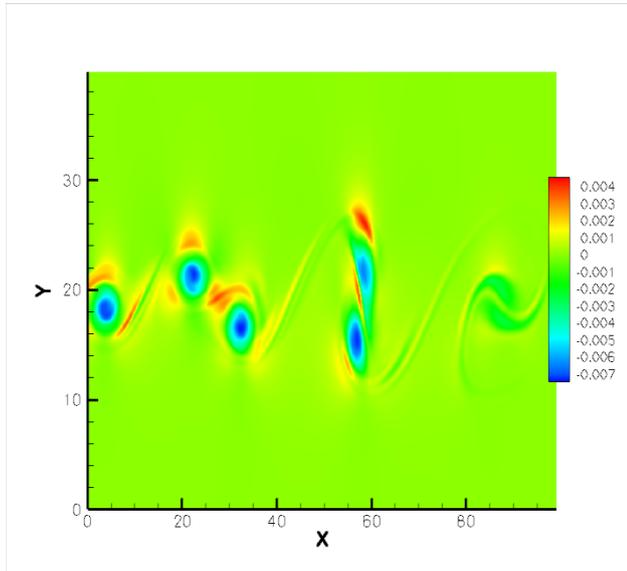
**Fig. 18** Sound source of spatial-developing mixing layer modeled with exponential decay.  $\tau = 0.0134$ .
