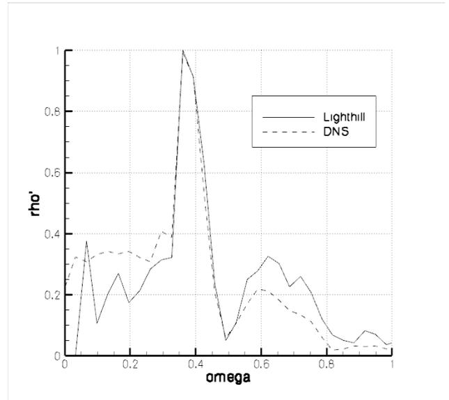
**Fig. 14** Comparison between Lighthill's analogy and DNS in frequency domain for Mach 0.1.
