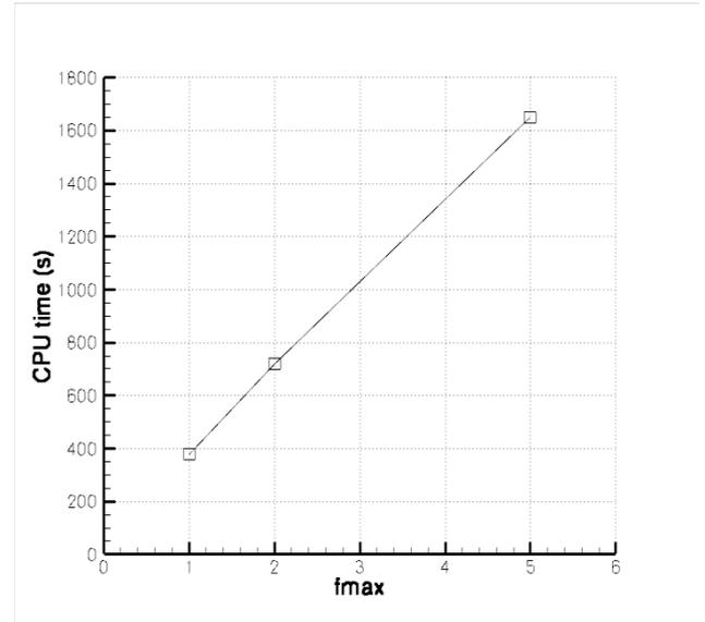
Fig. 11 CPU time dependence with frequency range.
