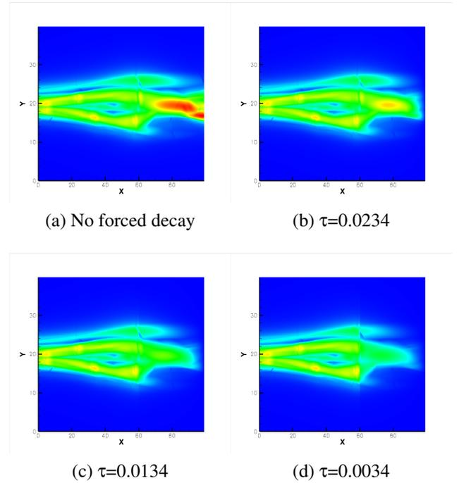
Fig. 17 Source envelope of a spatial-developing mixing layer for different  $\tau$ .
